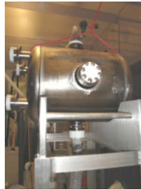
Figure 1: Orientation of HWR for first BCP etching set-up.
