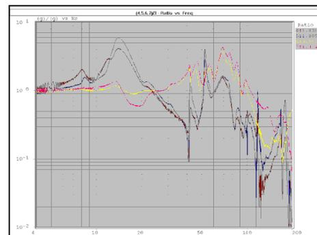
Figure 11: Resonance frequencies measured on cavity AC138.
