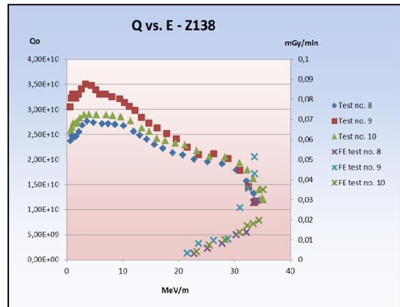
Figure 14: Q vs. E curve with Fe onset of test no. 8, 9 and 10.
