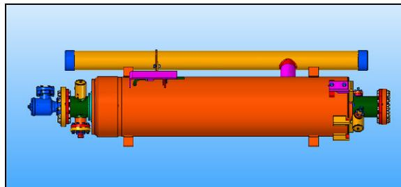
Figure 1: XFEL cavity in helium tank full equipped.
