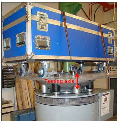
Figure 8: Cavity Z138 packed in transport case with different foam damping elements and rigged on simulator.
