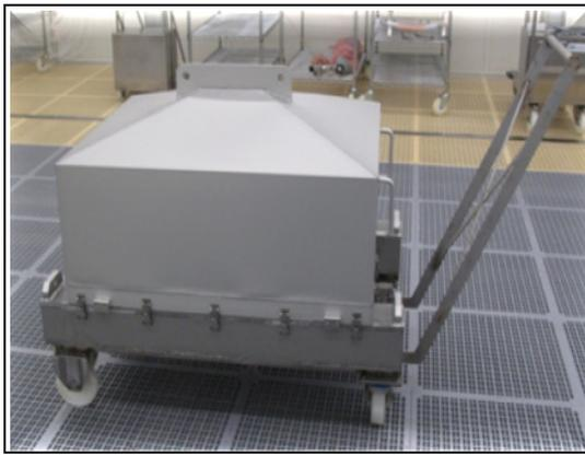
Figure 3: BQU located on a transport trolley and covered by transport hood.
