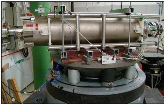
Figure 7: Cavity C24: installed into a handling frame and fixed directly on the vibration table without any damping elements.
