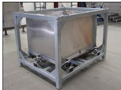
Figure 6: BQU transport frame with steel wire dampers.
