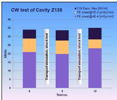
Figure 13: RF test results before, in-between and after transport tests.
