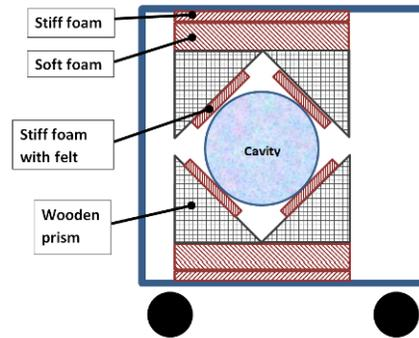
Figure 5: Foam concept of the transport case.
