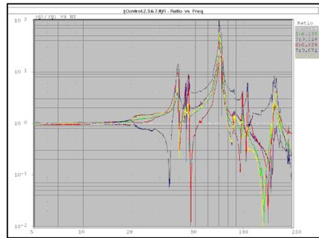
Figure 9: Resonance frequencies measured on cavity C24.
