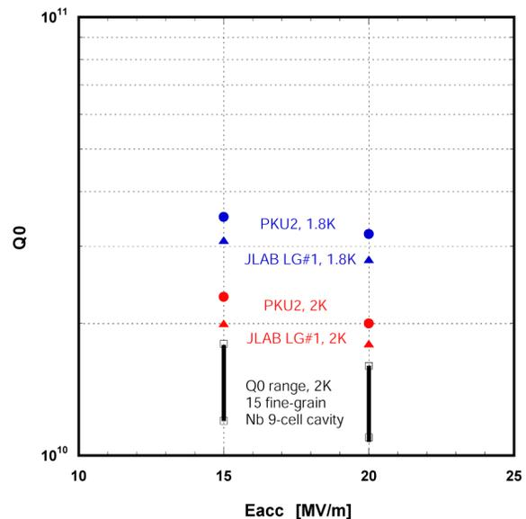
Figure 6: Comparison of  $Q_0$  values of 1300 MHz large-grain 9-cell niobium cavities to those of 1300 MHz fine-grain 9-cell niobium cavities similarly processed.
