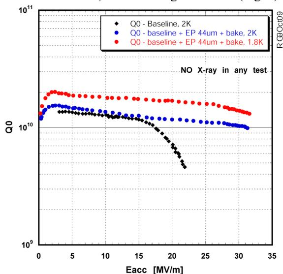
Figure 1: Test results of 1497 MHz 7-cell fine-grain niobium cavity HG008.
