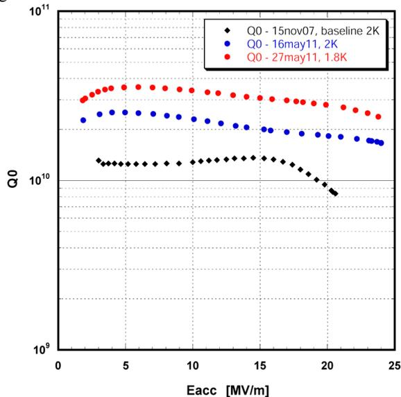
Figure 2:  $Q(E_{\text{acc}})$  curves of 9-cell large-grain niobium cavity JLAB LG#1 following an ILC-style final treatment including vacuum furnace high temperature heat treatment, light EP and in-situ low temperature bake. Test results at 2 K and 1.8 K are shown, along the baseline result at 2 K after BCP only and prior to any EP.
