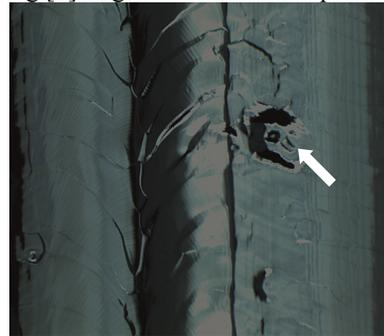
Figure 4: A pit of ~2mm in diameter (arrow) near the equator electron beam welding joint of the cell#1. Similar defects are observable in equator weld regions of all cells.
