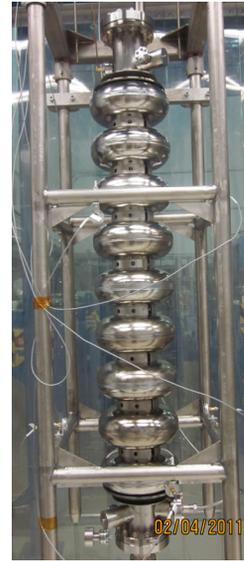
Figure 3: 9-cell large-grain niobium cavity PKU2.
