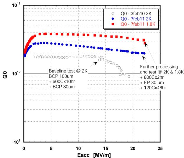
Figure 5:  $Q(E_{acc})$  curves of 9-cell large-grain niobium cavity PKU2 following an ILC-style final treatment including vacuum furnace high temperature heat treatment, light EP and in-situ low temperature bake. Test results at 2 K and 1.8 K are shown, along the baseline result at 2 K after BCP only and prior to any EP.
