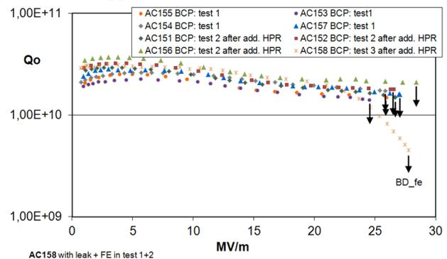
Figure 3: Final  $Q_0(E_{acc})$  performance at 2 K after BCP treatment. All cavities are limited by thermal breakdown; AC158 shows breakdown with strong x-rays (BD\_fe).
