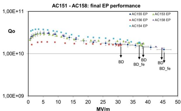
Figure 5: Final  $Q_0(E_{acc})$  performance at 2 K after EP treatment.
