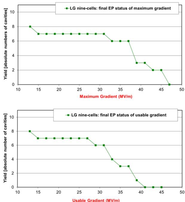
Figure 6: Yield of maximum and usable gradient in the final state after EP treatment in absolute numbers of cavities.
