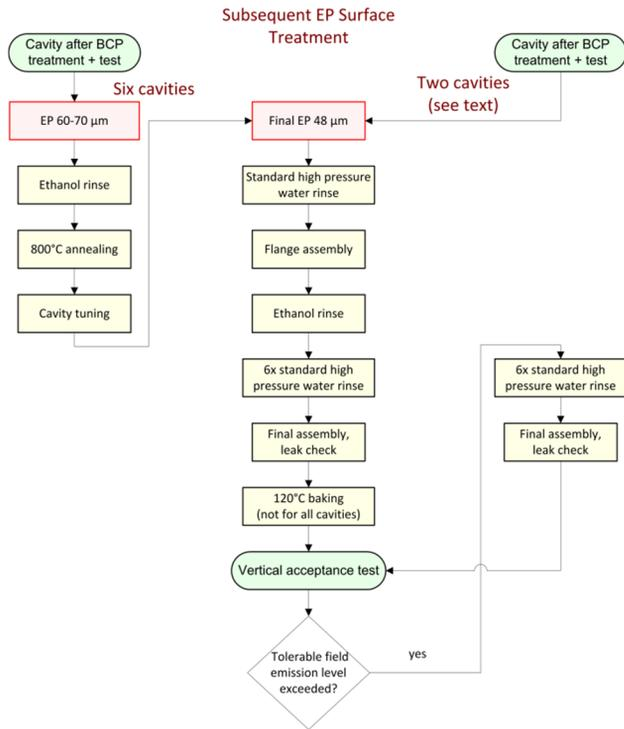
Figure 2: Flow scheme of subsequent EP treatment.
