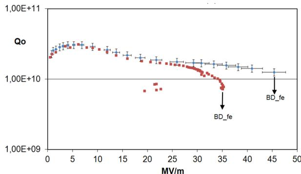
Figure 7: First and final  $Q_0(E_{acc})$  performance of nine-cell cavity AC155 at 2 K after EP treatment. Notice the Q-switches at around 30 MV/m down to (18 – 24) MV/m at  $Q_0$  below  $10^{10}$ .
