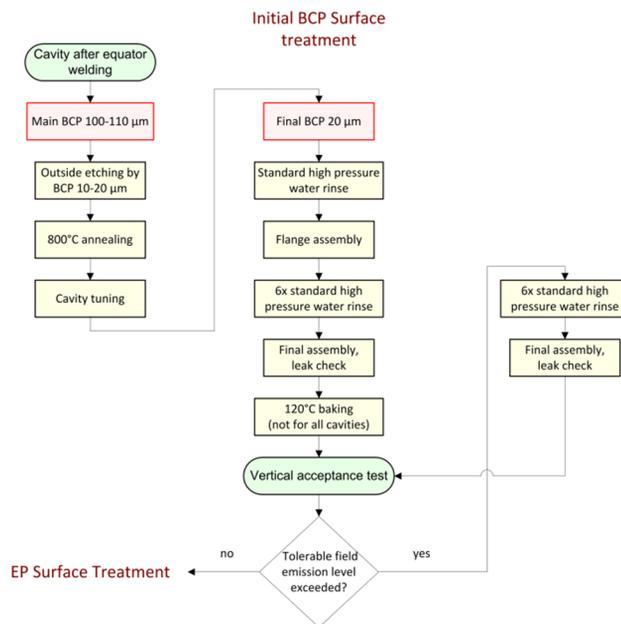
Figure 1: Flow scheme of BCP treatment.
