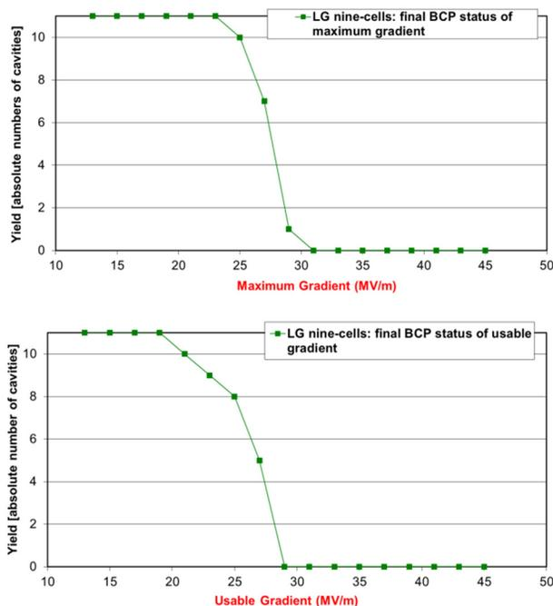
Figure 4: Yield of maximum and usable gradient in the final state after BCP treatment in absolute numbers of cavities.
