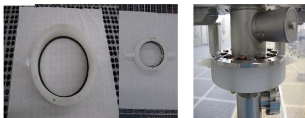
Figure 5: View on the rinsing set up/ left side: split rings for power- and beam pipe flanges / right side: rinsing set up installed to beam tube cavity long side.
