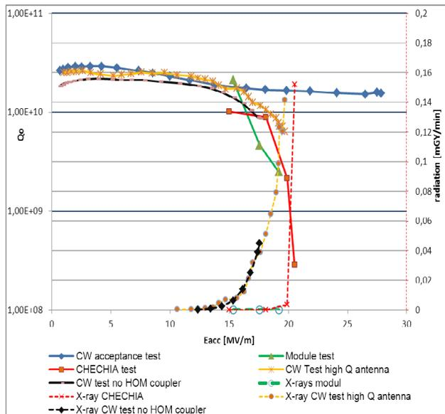
Figure 7: RF Test results of Cavity AC127.
