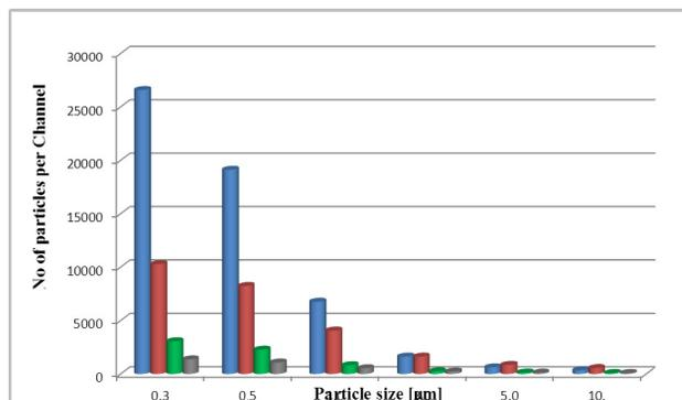
Figure 4: Test results of rinsing of beam pipe slit [Blue-Reference data of polluted slit; Red- Standard ultrasonic rinse; Green- Rinsed via split ring with ethanol; Grey- rinsed via split ring with ultra-pure water.
