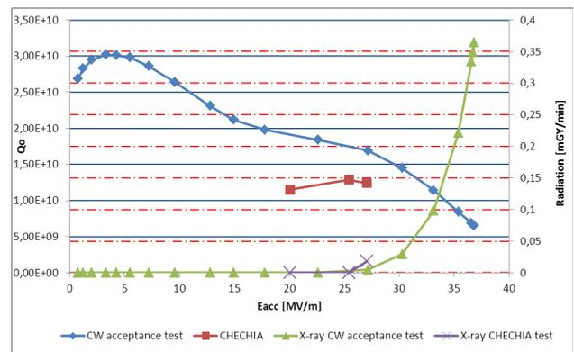
Figure 1: RF Test results of cavity AC 113.
