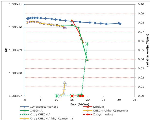
Figure 6: RF test results of Resonator Z88 analysis
