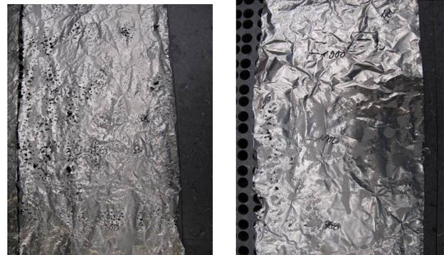
Figure 2: left side: US pattern on Al foil @ level 600 mm from bottom/ right side US pattern on Al foil @ level 1900 mm from bottom.
