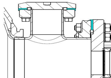
Figure 3: Cross section seals (beam tube long side).
