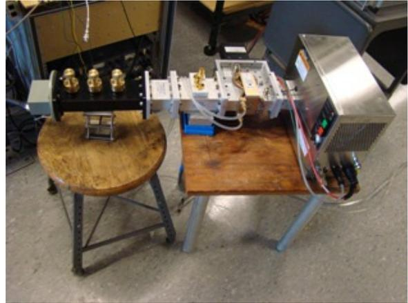
Figure 4: Microwave power supply with circulator, tuner and power meter.
