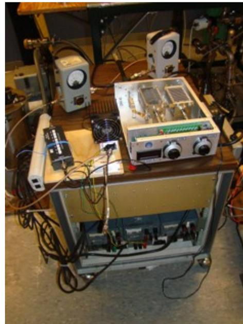
Figure 5: Radio frequency power supply with matching network and power meter.
