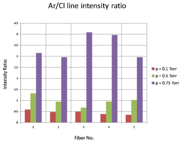
Figure 6: Relative intensity of argon and chlorine lines.
