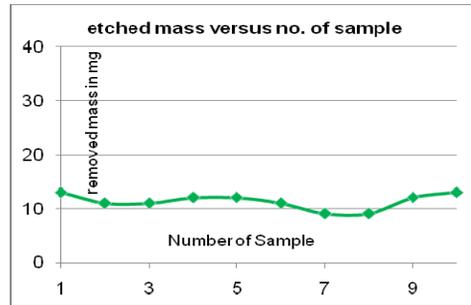
Figure 8: Material removed by plasma etching as a function of sample position on cavity surface.
