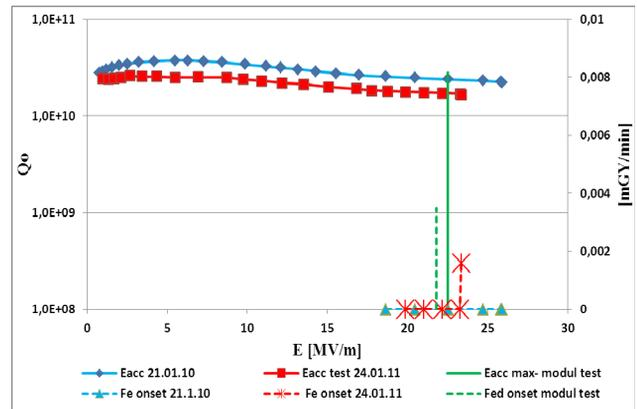
Figure 5: Test results of cavity Z140 before (blue lines), during (green lines) and after (red lines) application in module.
