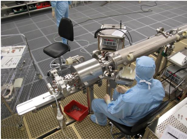
Figure 2: View on the BQU during preparation for disassembly (left side flushing unit installed to gate valve)
