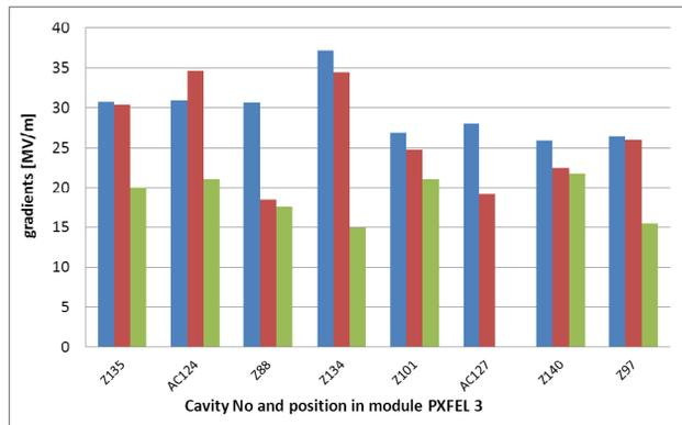
Figure 3: Test results of PXFEL3 module on CMTB. (Blue bars - maximal gradient in vertical test; Red bars - maximum gradient in module test; Green bars - X-ray onset gradient in module test).
