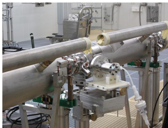
Figure 1: View on Cavity connection in preparation for disassembly.
