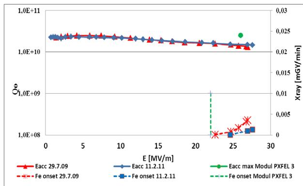
Figure 4: Test results of cavity Z101 before (blue lines), during (green lines) and after (red lines) application in module.
