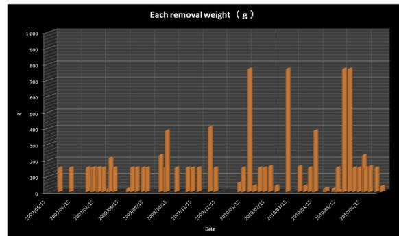
Figure 5: Each removal weight of niobium from cavity for the 59 EP-processes.
