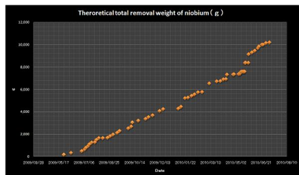
Figure 6: The accumulated removal weight of niobium calculated from the total charge (integrated current) of EP processes vs. date.
