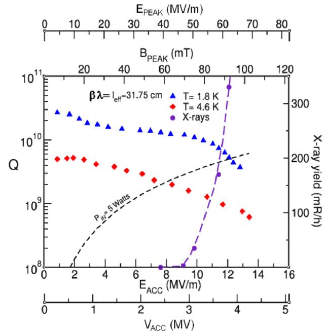
Figure 5: A Q-curve of the new prototype 72 MHz QWR cavity processed at ANL for the ATLAS Intensity Upgrade.
