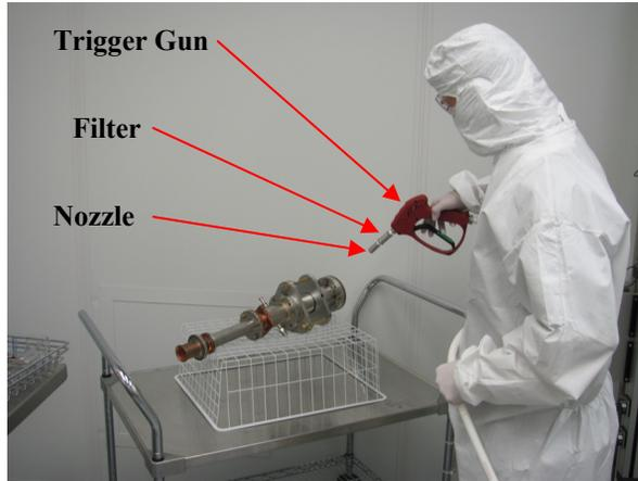
Figure 4: A hand HPR wand allows the operator to rinse the hardware, rather than blowing the hardware off with N<sub>2</sub>, saving time. A 0.5 μm filter is located just before the nozzle of the tool, and removes possible particulates from the trigger mechanism.
