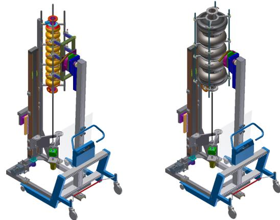
Figure 2: The tool can accommodate virtually any type of cavity. Shown are a 650MHz 5-cell elliptical cavity (bottom right), a 1.3 GHz 9-cell elliptical cavity (bottom left), and a 72MHz quarter wave resonator cavity (top).
