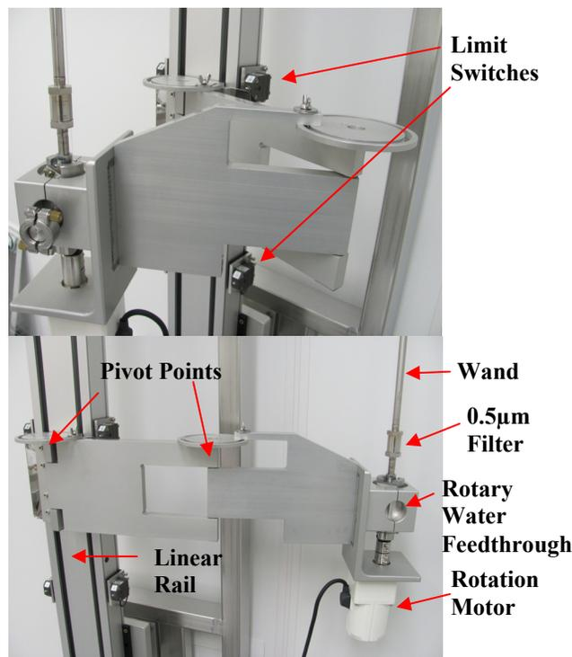
Figure 1: Mounting the HPR rinse wand on a 2-hinged arm allows for the rinsing of any port within the 26" radius.
