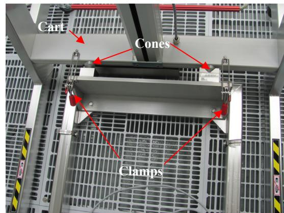
Figure 3: A mounting block and tie down clamps for the cart ensures repeatable positioning of the cavity. This also provides the ability to move the cavity about the room, rinse it, and assemble it without removing it from the cart.
