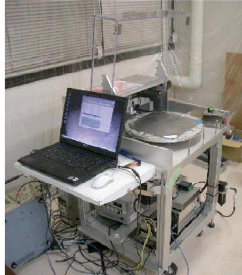
Figure 1: Eddy Current Scanner.
