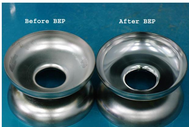
Figure 4: Photos of Nb dumbbells polished by BEP via the shaped cathode of Fig. 3 a) before BEP treatment, b) after BEP treatment.
