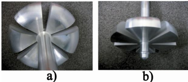
Figure 3: Photos of the shaped cathode fabricated at JLab according to the design from PKU. a) top view, b) side view.
