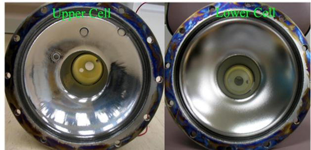
Figure 7: Photos of the upper and lower cells of the demountable cavity after treating by BEP using a wheel shape cathode.
