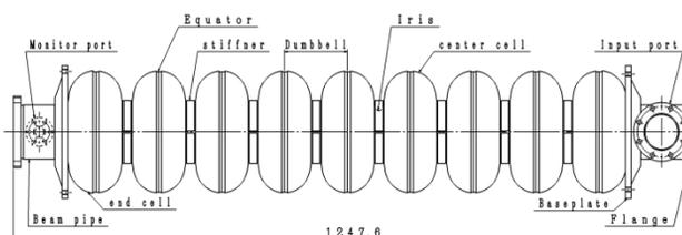
Figure 1: 9-cell superconducting cavity without HOM couplers.
