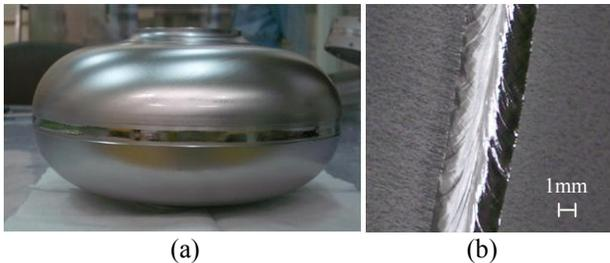
Figure 2: (a) Test pieces of equator welding, (b) Typical inner picture of the EBW seam at equator.
