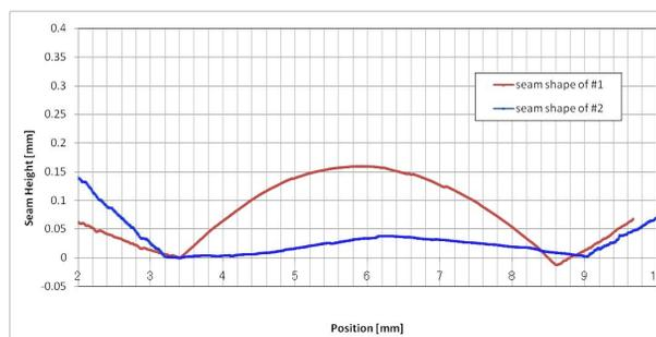
Figure 5: Equator welding seam comparison. The red line shows first cavity's seam form (#1) and the blue line shows improved seam form (#2).
