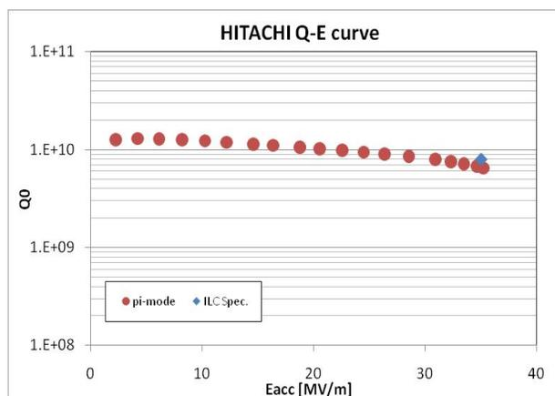
Figure 4: Q-E curve for our first 9-cell cavity.
