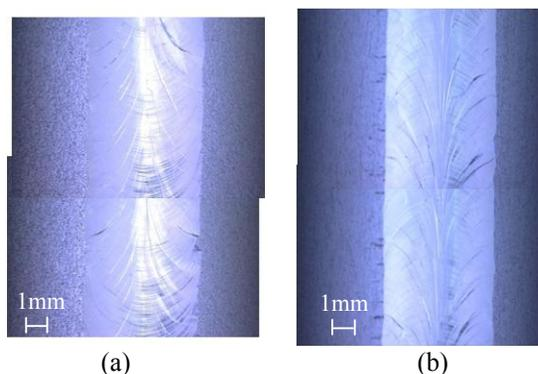
Figure 6: Equator welding seam comparison by optical camera. (a) Improved #2 seam, (b) #1 seam.
