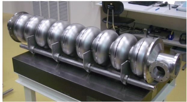
Figure 3: Completed 9-cell cavity.
