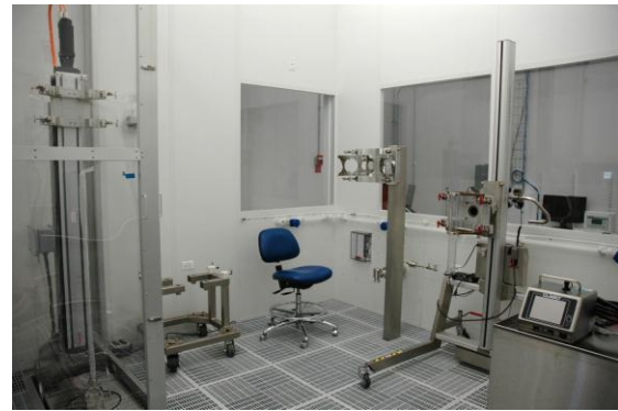
Fig 7: ISO Class 4 cleanroom with HPR tool.
