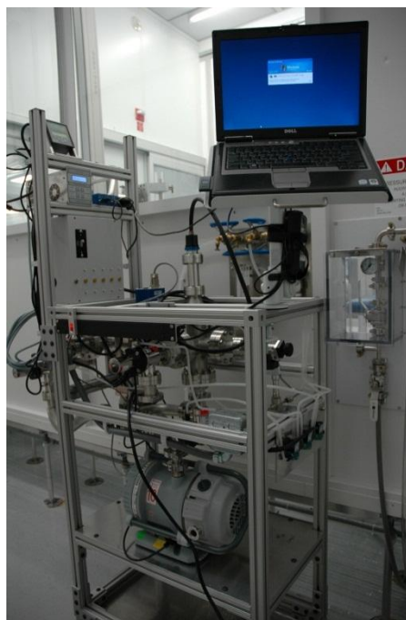
Figure 9: UHV Dry Pumping and Venting System
