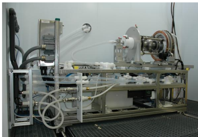
Figure 3: Horizontal electropolishing tool shown with a single cell Tesla-type cavity.
