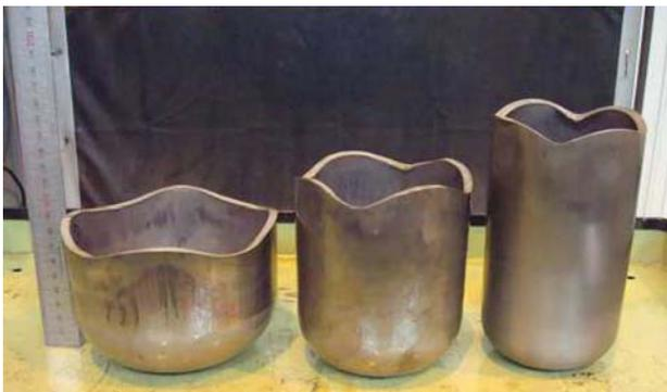
Figure 9: Fabricating process of long cups. (Left: after 1<sup>st</sup> deep drawing, Center: after 2<sup>nd</sup> deep drawing, Right: after 3<sup>rd</sup> deep drawing).
