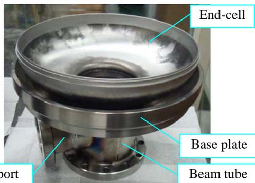
Figure 6: End-group by the side of input port.
