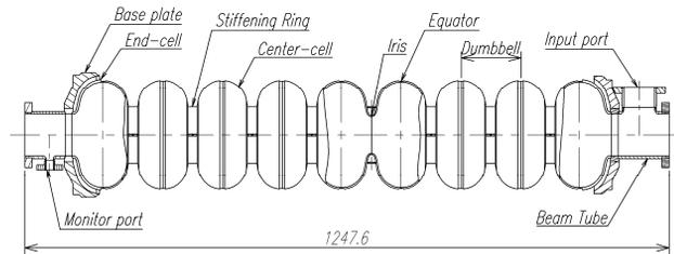
Figure 1: Drawing of 9-cell superconducting cavity without HOM couplers.
