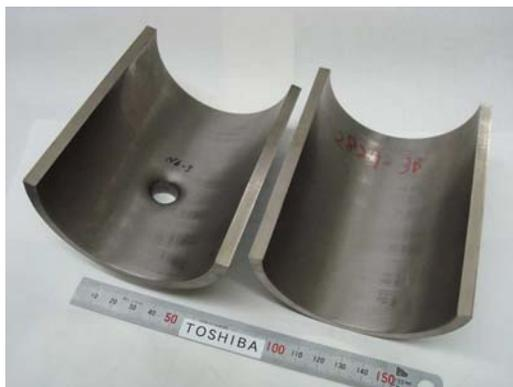
Figure 8: Half-pipes for the beam tube of the 1<sup>st</sup> cavity.
