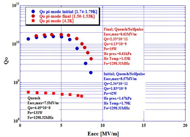
Figure 7: RF test result of the 9-cell cavity. Low current density EP-II (20  $\mu\text{m}$ ) with  $\text{N}_2$  gas flow, rinse with ultra-pure water (1.5 hrs), detergent rinse with FM\_20 of 2 % (50  $^{\circ}\text{C}$ , 2 hrs), HPR (10 hrs).
