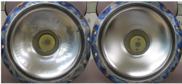
Figure 9: The CCD pictures of single cell cavity treated by EP process with the wheel cathode 3. Left one is the upper half cell; right one is the lower half cell.
