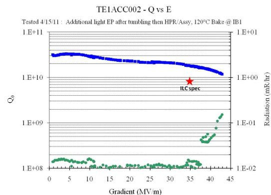
Figure 1: Cold test results for TE1ACC002.
