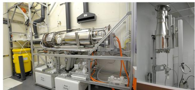
Figure 5: Prototype QWR mounted in the new low- $\beta$  EP tool (left) and in the new HPR tool (right).
