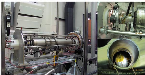
Figure 3: Dressed cavity mounted in EP tool (left). Anode connection (upper right) and thermometry (lower left).
