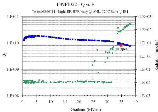
Figure 2: Cold test results for TB9RI022.
