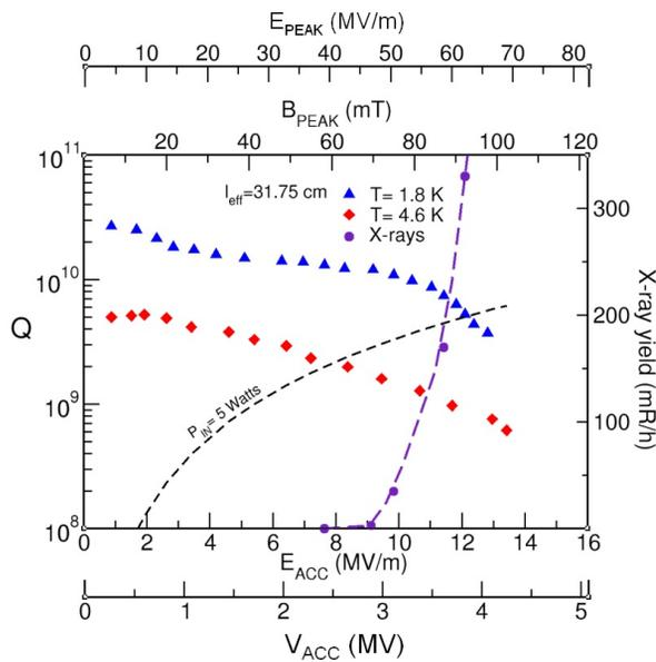
Figure 6: Cold test results for the prototype QWR.
