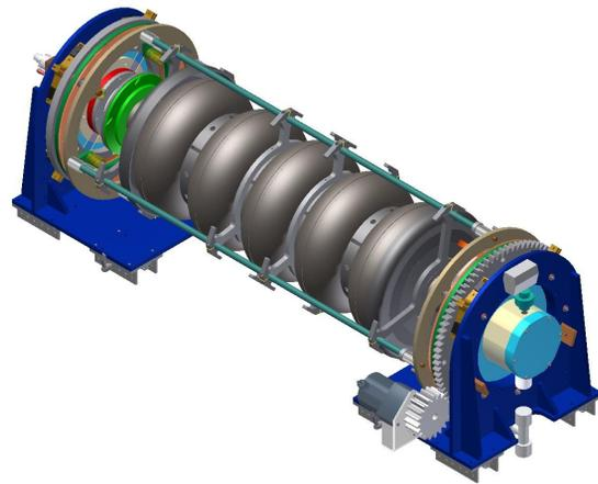
Figure 7: Complete 3-D model of the low- $\beta$  EP tool adapted for 650 MHz elliptical cavities.
