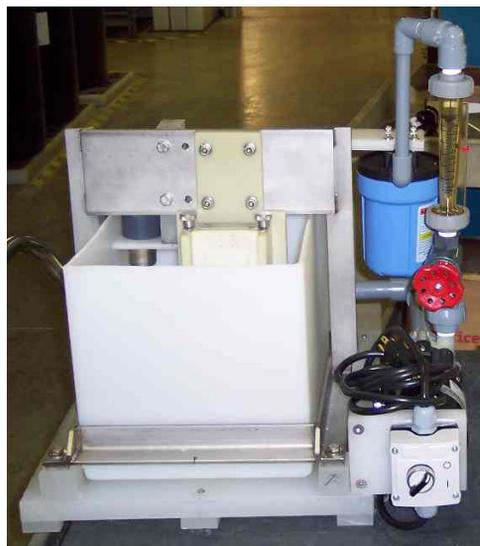
Figure 2: Bench-scale apparatus for electropolishing niobium coupons for process development activities.
