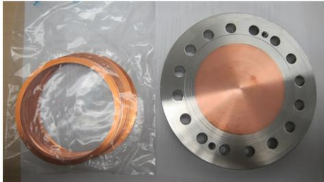
Figure 10: Image of Cu gasket and Cu/SUS flange.
