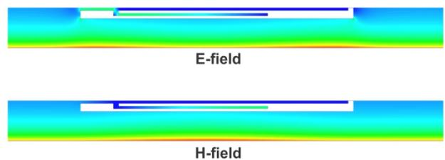
Figure 7: Electric and magnetic fields in geometry with choke-shield.
