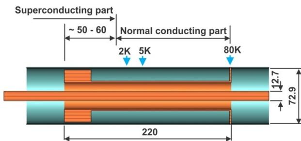
Figure 3: Slot with step-shield. Coupler has 50 times less 2K-5K cryogenic loss then conventional coupler.
