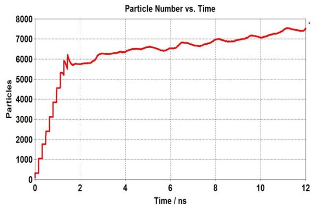
Figure 12: Number of particles vs. tame for 128 kW of RF power. Power is above of multipactor threshold.
