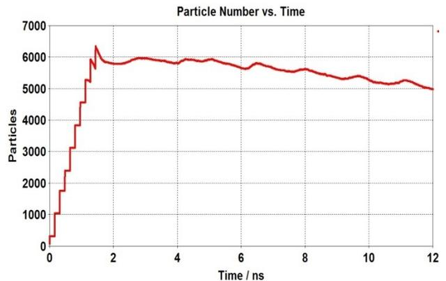
Figure 11: Number of particles vs. tame for 64 kW of RF power. Power is below of multipactor threshold.
