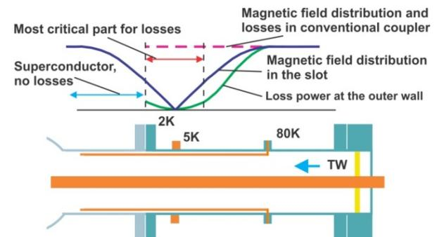
Figure 2: Gain can be much more if low temperature area is placed near minimum of magnetic field.
