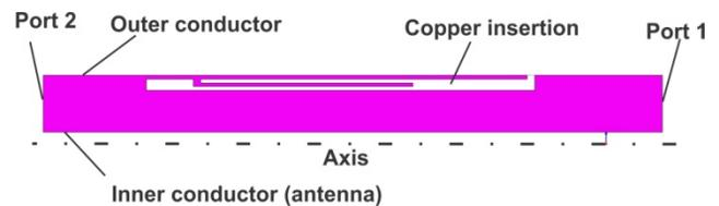
Figure 6: Geometry with choke-shield.
