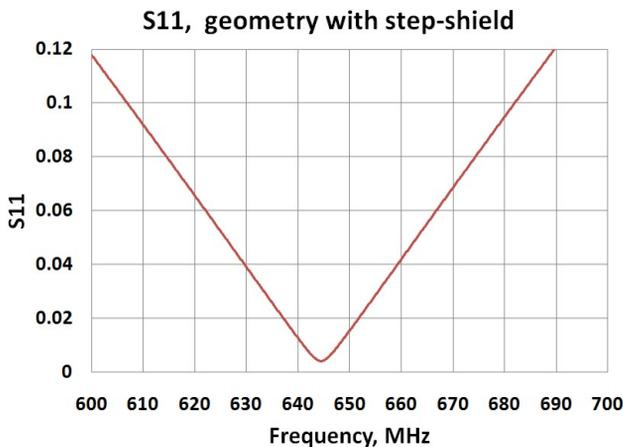
Figure 4: Passband of coupler with step-shield.
