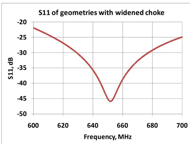
Figure 9: Passband of geometries with widened choke.
