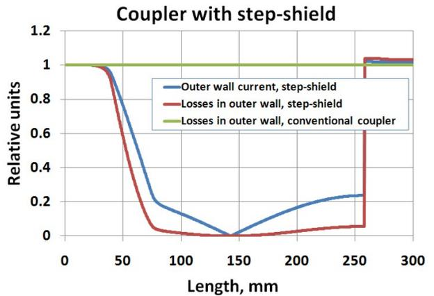
Figure 5: Geometry with step-shield. Distributions of current and losses along surface of outer pipe.
