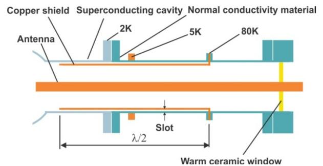
Figure 1: Simple RF shield:  $1/2\lambda$  copper pipe with single mechanical-thermal contact with stainless steel outer pipe.
