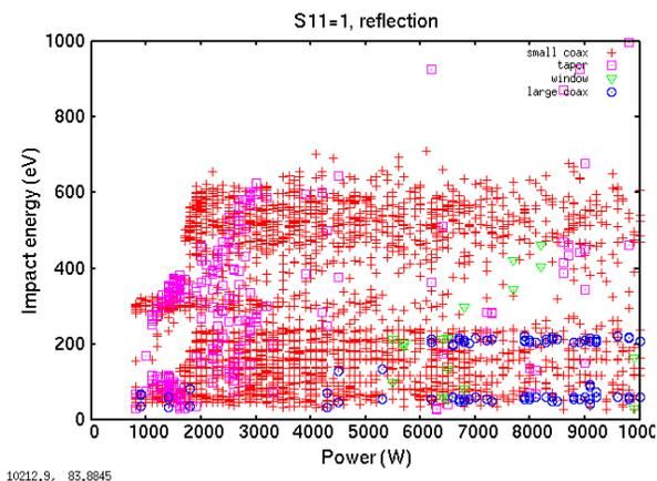
Figure 2: Calculated impact energy of multipacting bands of the FRIB FPC as a function of input power.
