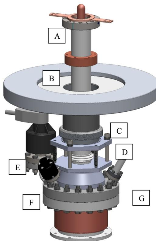
Figure 1: FRIB Prototype Fundamental Power Coupler. (A) 4K intercept, vacuum break and RF seal, (B) 38 K intercept, (C) Bellows for thermal contraction (D) Bellows for coupling adjustment, (E) Cold Cathode Gauge, (F) Spark Detector, (G) E-probe.
