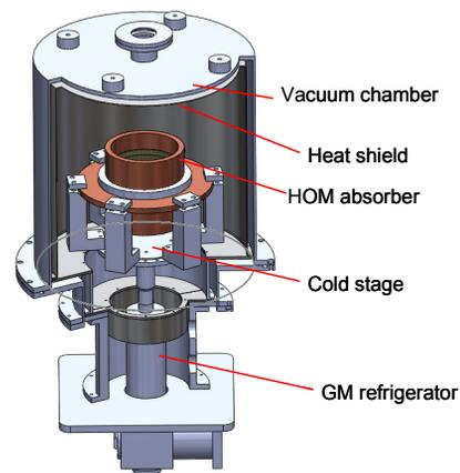
Fig. 7: Schematic view of cooling cycle setup for HOM absorber model with HIP ferrite.
