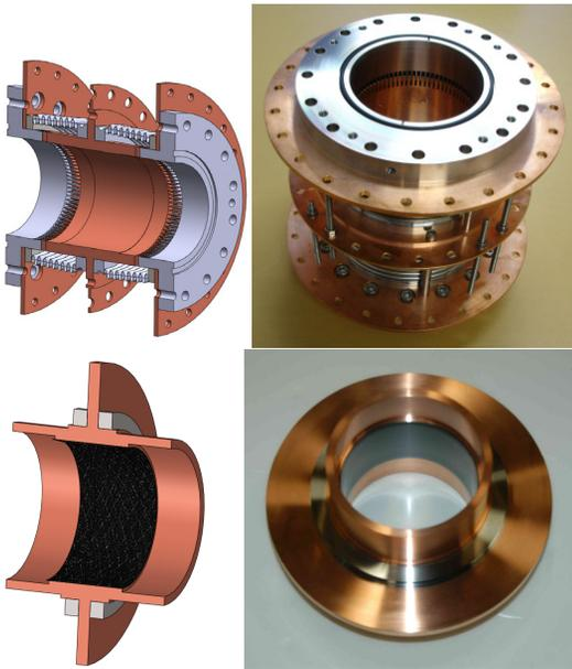
Fig. 2: Schematic views and photographs of HOM absorber models without HIP ferrite (upper) and center part with HIP ferrite (lower).
