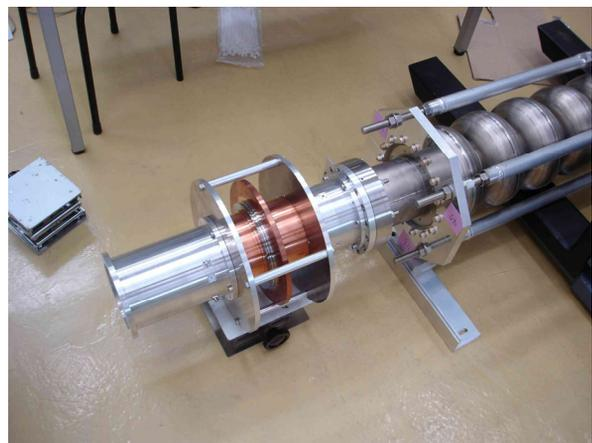
Fig. 5: Setup of HOM absorption measurement with our 9-cell ERL model cavity.
