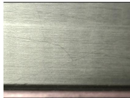
Fig. 8: Linear cracks observed near the tapered ferrite edge.
