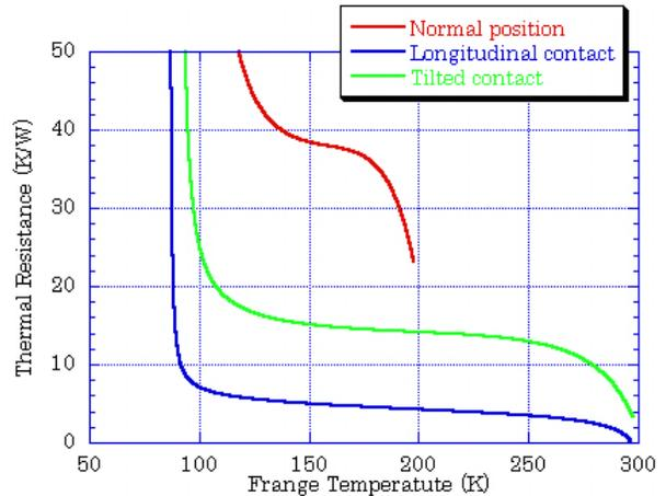
Fig. 3: Thermal resistances in the normal position, with longitudinal and tilted contact.
