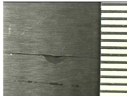
Fig. 9: Trail of chipped-off piece (left) and 1mm-scale (right).
