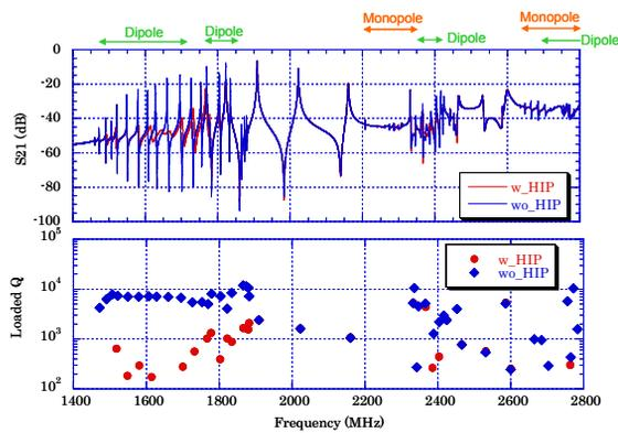
Fig. 6: HOM peaks and Q-values with and without HIP ferrite.
