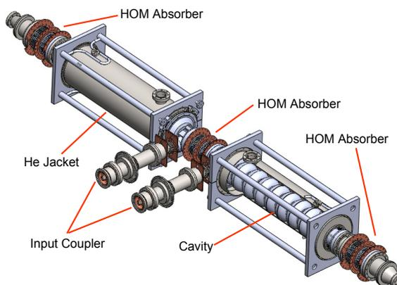
Fig. 1: Layout of HOM absorbers in the cryomodule.
