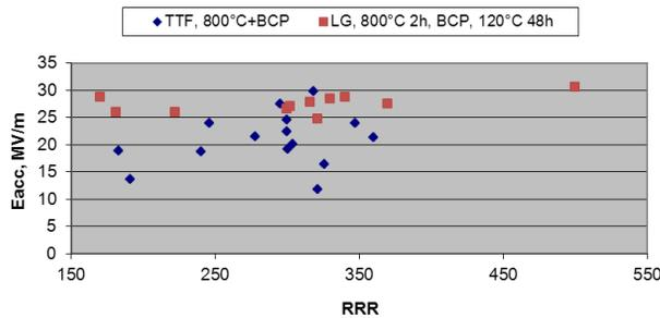
Figure 2: Maximum  $E_{acc}$  measured in fine-grain (blue diamonds) and large-grain (red squares) cavities treated in a similar way, as a function of the RRR of the Nb. The figure is from Ref. [4]
