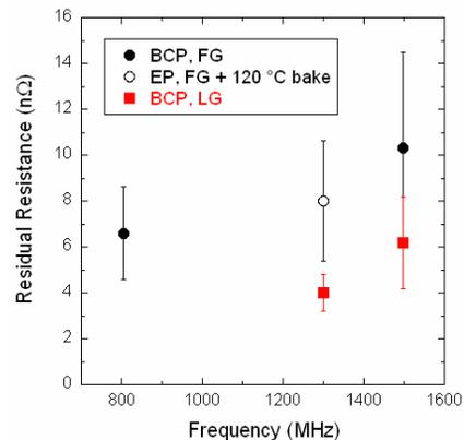
Figure 3: Residual resistance values obtained from the low-field  $Q_0(2.0$  K) for fine-grain (FG) [8] and large-grain (LG) cavities at different frequencies. The figure is from Ref. [7].
