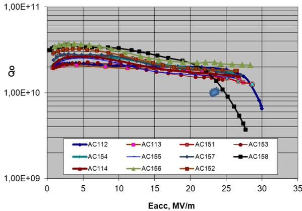
Figure 1:  $Q_0(E_{acc})$  measured at 2 K at DESY for 11 1.3 GHz 9-cell cavities manufactured by ACCEL and treated by BCP. The  $Q_0$  degradation at high field for cavities AC158 and AC112 is due to field emission and  $Q$ -drop (AC112 was not baked at 120 °C), respectively. The star symbol indicates the requirement for the XFEL project. The figure is from Ref. [4].
