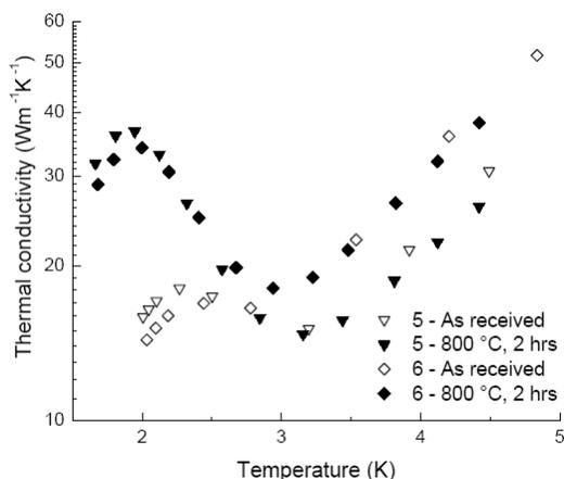
Figure 5: Thermal conductivity as a function of temperature measured on two bi-crystal samples before and after heat treatment at 800 °C for 2 h. The Ta content is 1322 wt-ppm and 523 wt-ppm for samples 5 and 6, respectively. The figure is taken from [19].
