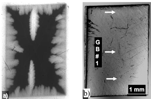
Figure 4: Magneto-optical image showing flux penetration at the GB at 6 K and 80 mT magnetic field, applied nearly parallel to the GB plane (a). The optical image of the bi-crystal sample is shown in (b). The figure is from [15].
