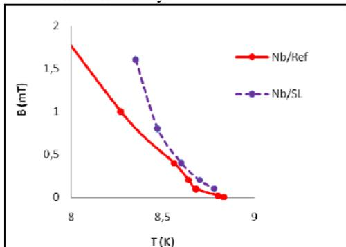
**Figure 7: First penetration field for niobium in the Reference (continuous) and in the SL (dotted) (detail of the low field part of figure 5). The first penetration of vortices in niobium covered with a NbN layer (SL) appears at a apparent field values higher than the same niobium layer when directly measured in Reference. The Nb layer is effectively screened by the NbN layer, even in the perpendicular field configuration.**
