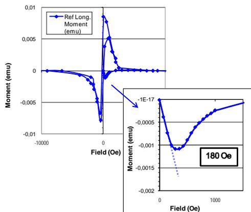
**Figure 1: Magnetization curves at 4.5 K for the Reference sample (250 nm Nb): longitudinal moment at low field and determination of the first penetration field  $B_p$ . As expected for an isotropic superconductor,  $B_p$  is found to be the same in the transverse direction (not shown here).**
