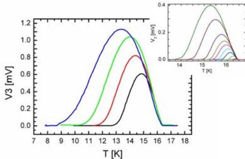
**Figure 3:** Set of third harmonic signals measured for an increasing series of AC magnetic field. Insert show an expansion of the scale for low fields. For each field one can determine the temperature of the first penetration of vortices (left-hand threshold of the V3 curve) and reconstruct the  $B_{C1}$  vs T curve.
