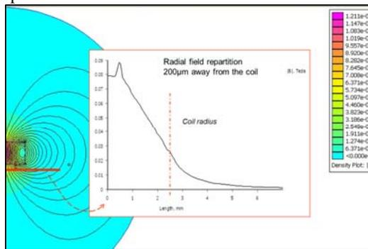
**Figure 4:** Field repartition for a 5 mm diameter coil. Inset shows the radial repartition 200  $\mu\text{m}$  away from the coils (approximate position of the sample is expected to be closer to the coil:  $\sim 60\mu\text{m}$ ).
