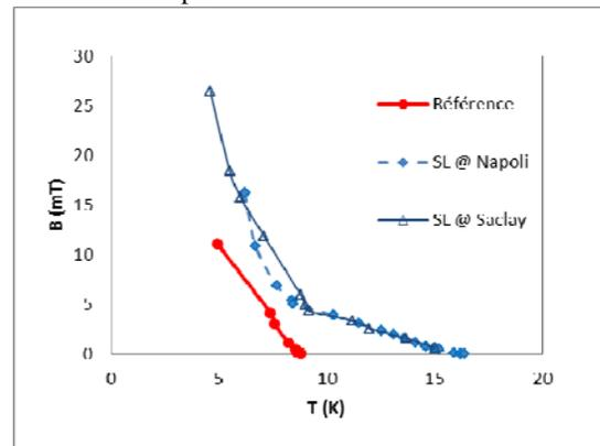
**Figure 6:** First penetration field for the Reference sample (red, circles) and the SL samples (blue, diamonds for Napoli experiment, triangles for the Saclay experiment) as determined with the third harmonic local probe. Around 6K, The first penetration of vortices in SL appears at a field value about twice the Reference's one.
