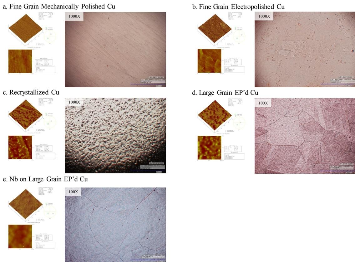
Figure 1: Representative AFM and Hirox images for the substrate preparation steps and ECR Nb on large grain Cu.
