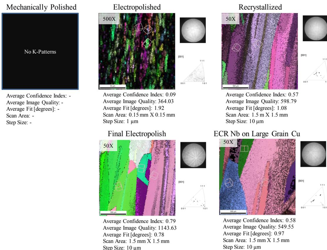
Figure 3: EBSD characterization of Cu substrates at each processing step and a typical ECR Nb deposition on the final electropolished surface (Maps cleaned up with neighbour CI correlation of 0.2%, represented by the dark pixels).
