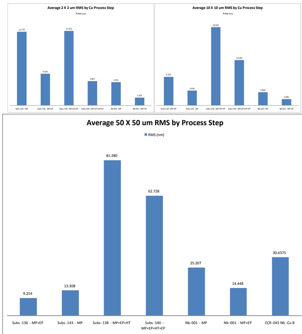
Figure 2: Average AFM RMS (nm) for Substrate Preparation Steps by Scan Area.
