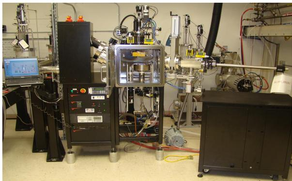
Figure 1: Vacuum chamber (PLD 5000) at the Jefferson Lab Facility Free Electron Laser, used for surface treatment on SRF Niobium disc.
