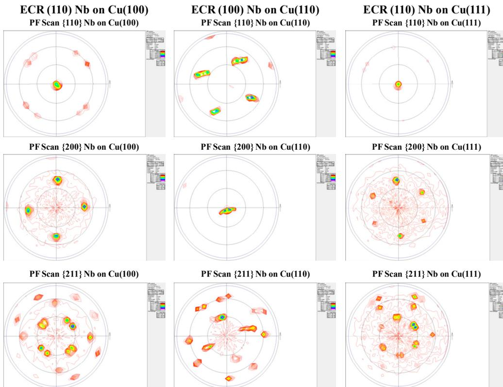
Figure 2: Pole figures for Nb(110), Nb(200), and Nb(211) are presented for each of the single crystal Cu orientations (100), (110), and (111).
