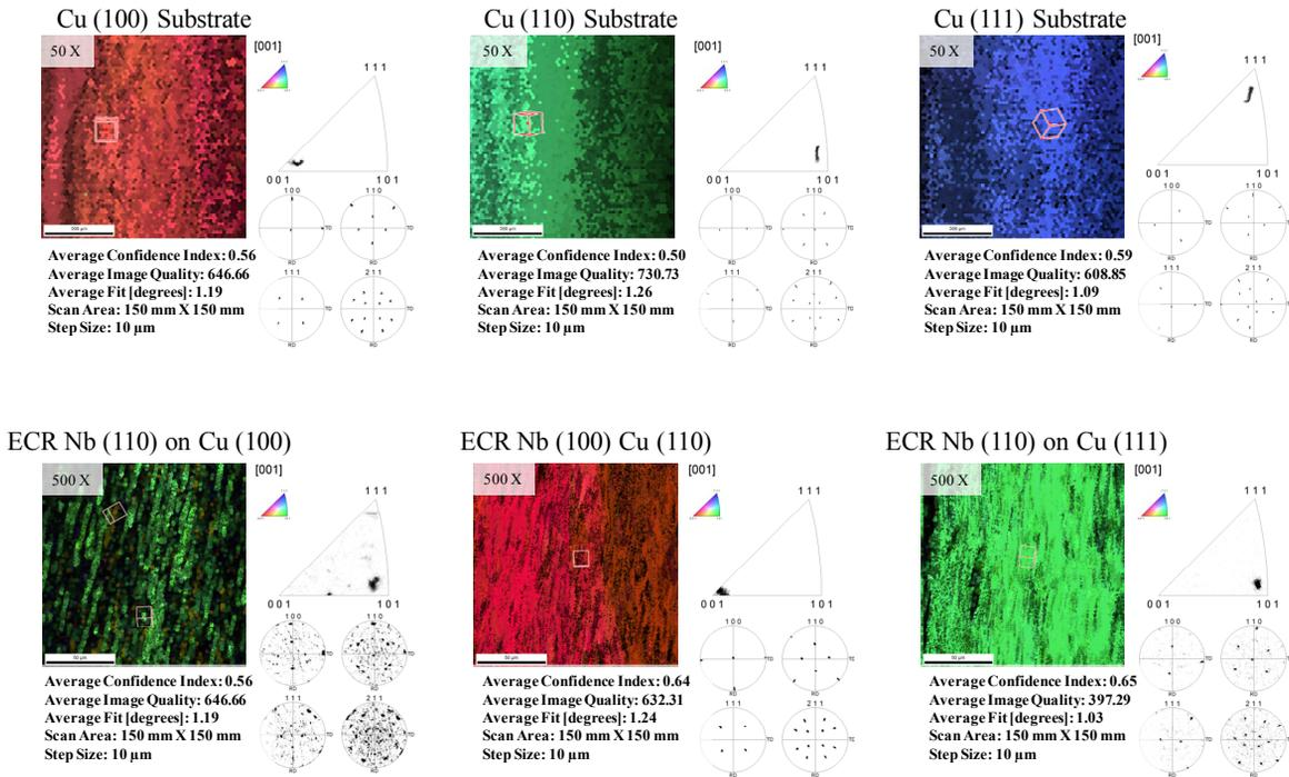
Figure 1: Top EBSD maps of Cu single crystal substrates with EBSD IPF and pole figures below. Bottom pane is EBSD for ECR Nb coatings on single crystal Cu orientations (maps post processed with neighbor confidence index (CI) of 0.2 and the EBSD map grey scale is based on a CI of 0.2%).
