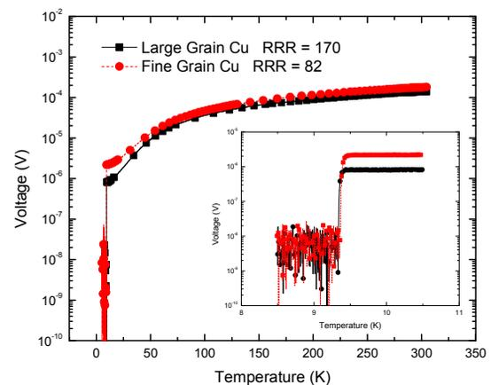
Figure 4: Resistivity versus temperature curves for ECR Nb on large and fine grain Cu. Large grain Cu substrate is the red dashed line with filled circles and fine grain substrate is the solid black line with filled squares.
