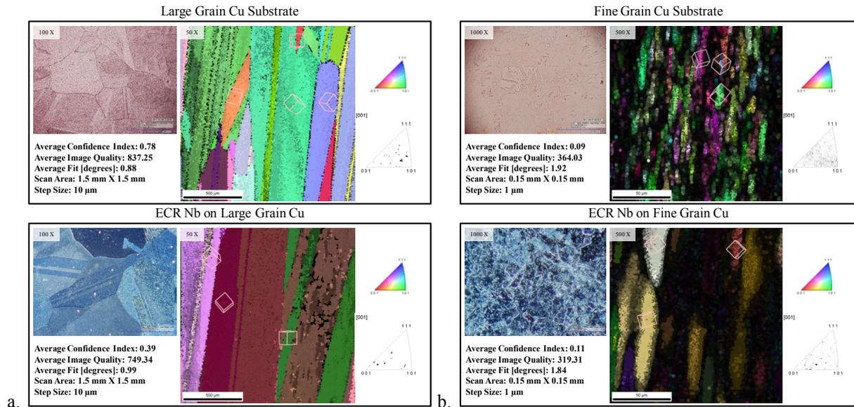
Figure 3: Hirox images and EBSD maps of large and fine grain Cu substrates and ECR deposited Nb thin films.
