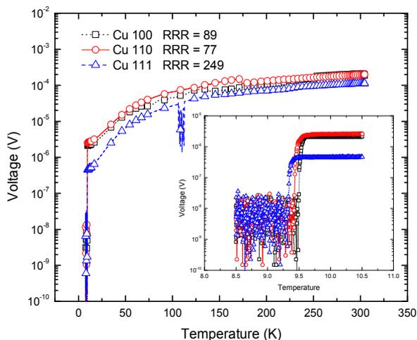
Figure 5: Resistivity versus temperature curves for ECR Nb on single crystal Cu orientations (100), (110), and (111). ECR Nb on (100) Cu is the dotted black line with open squares, ECR Nb on (110) Cu is the red solid line with open circles, and ECR Nb on (111) Cu is dashed blue line with open triangles.
