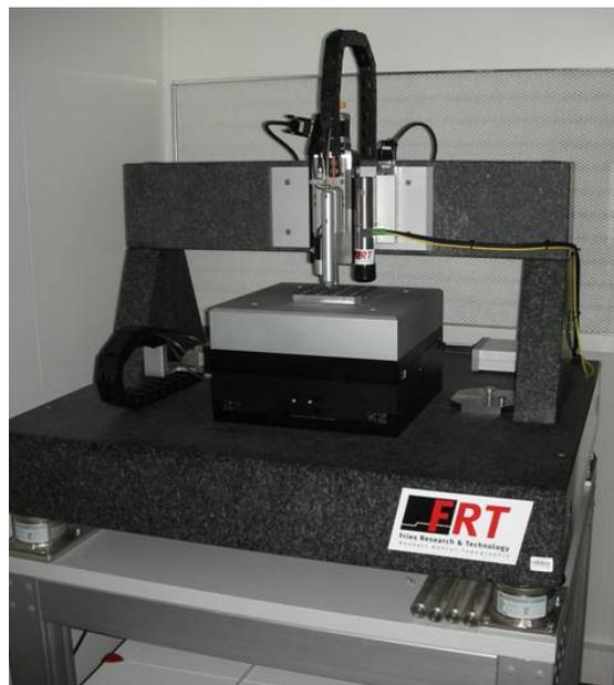
Figure 3: Optical profilometer with AFM.
