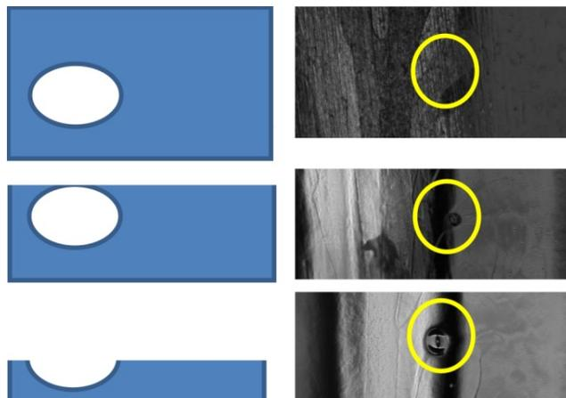
Figure 1: Defect uncovered by consequent EP and tracked by optical inspection (FNAL, D. Sergatskov).
