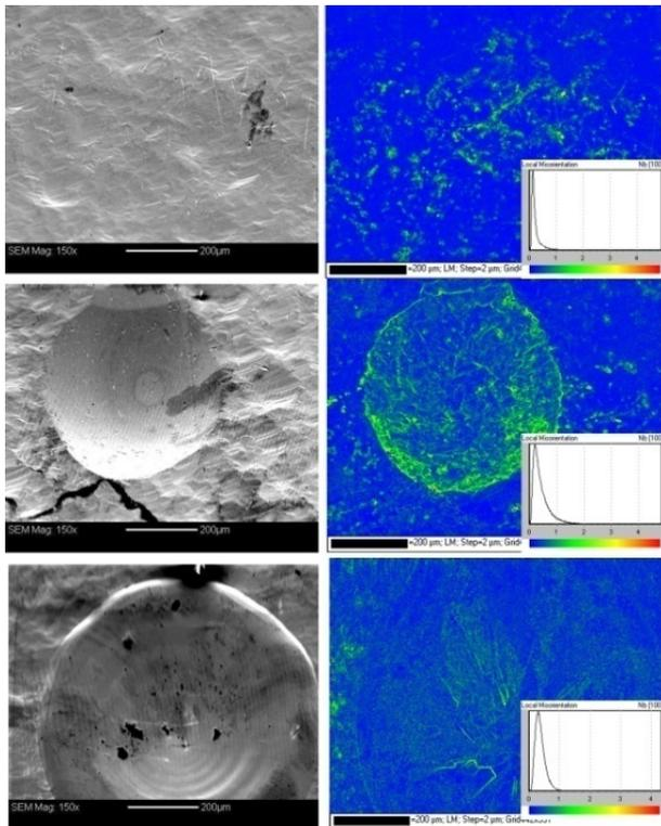
Figure 2: Electron microscope snapshots of initial surface, indent on the surface, remelted indent(left column). And concurrent local misorientation maps, showing stress amount persisting during each of the steps obtained by means of EBSD (left column).
