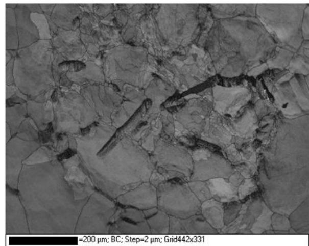
Figure 4: Contrast map of the HAZ underwent light etching obtained by means of EBSD.
