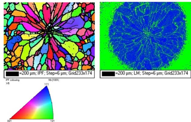
Figure 3: Orientation map and misorientation map for remelted zone in the absence of the artificial pit. Legend inclusion describes the color scheme for OM.
