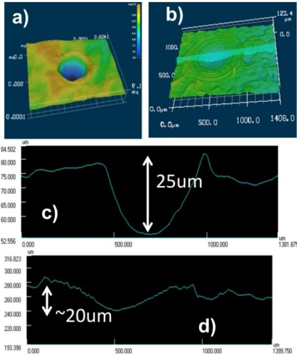
Figure 5: Laser confocal microscopy data. (a) 3D - indented pit, (b) HAZ after remelting. (c) 2D - indented pit, (d) HAZ after remelting.
