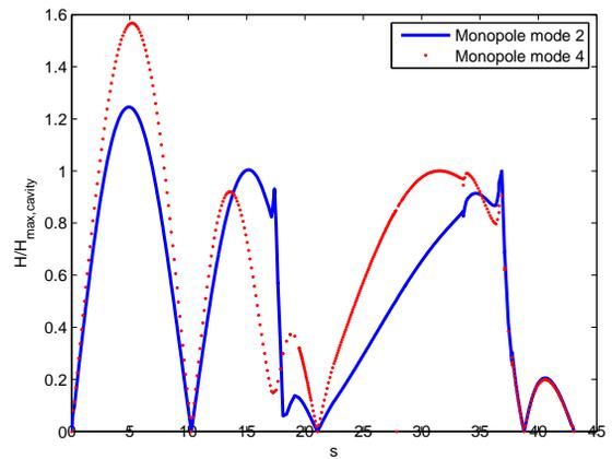
Figure 12: Normalized surface magnetic field along the sample plate and walls of the host cavity. Sample plate: s=0 to 10 cm. Host cavity: s=10 to 43 cm.
