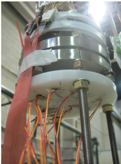
Figure 10: Sample plate thermometry system for TE pillbox cavity.
