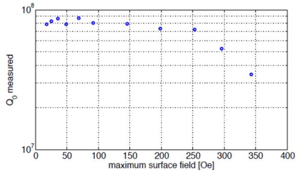
Figure 8: Q vs H for new niobium input coupler at 1.6K for TE pillbox cavity baseline niobium sample plate.
