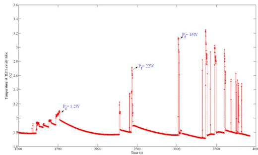
Figure 5: Heating observed during rf test with copper input coupler.
