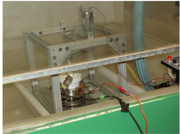
Figure 3: EP setup for TE cavities.
