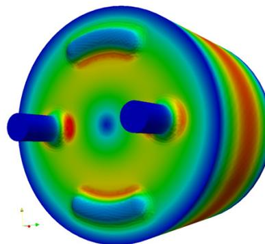
Figure 1: Surface magnetic field distribution of the  $TE_{011}$  mode of TE pillbox cavity.
