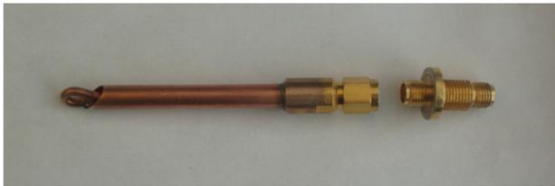
Figure 6: The copper input coupler and its SMA line connector feedthrough.
