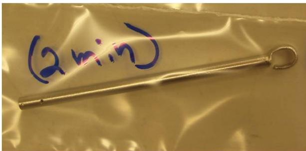
Figure 7: Niobium input coupler body after a light BCP.
