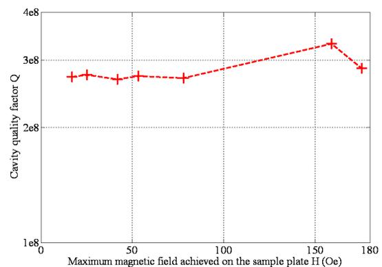
Figure 4: Q vs H for copper input coupler at 1.8K for TE pillbox cavity baseline niobium sample plate.
