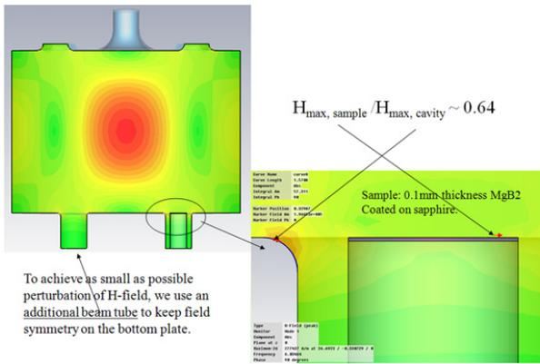
Figure 2: Symmetric ports on bottom plate enabling placing a sample on a sapphire rod in the high magnetic field region.
