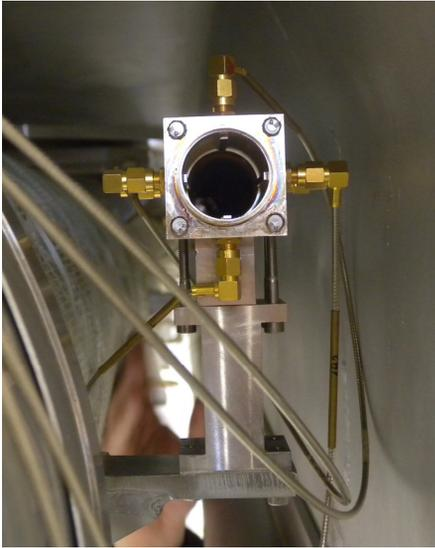
Figure 2: Stripline wire position pickup fixed to the He gas return pipe of the TESLA-style cryomodule.
