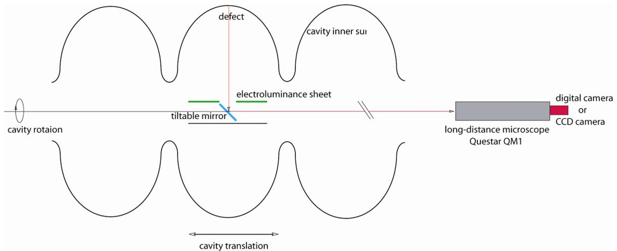
Figure 2: Principle of high-resolution SRF cavity inspection using a long-distance microscope.
