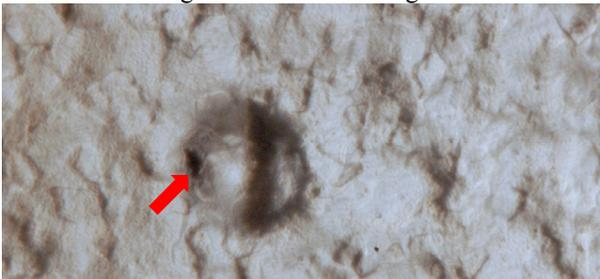
Figure 6: A circular defect with a  $\sim 10 \mu\text{m}$  core (indicated by arrow) discovered by JLab high-resolution SRF cavity inspection machine on a 9-cell cavity surface.
