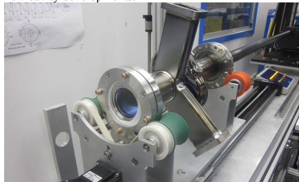
Figure 7: Inspection of a crab cavity being developed at JLab for ANL's APS upgrade project.
