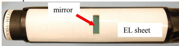
Figure 3: The mirror and electroluminescence sheet at the end of the mirror-bearing tube.
