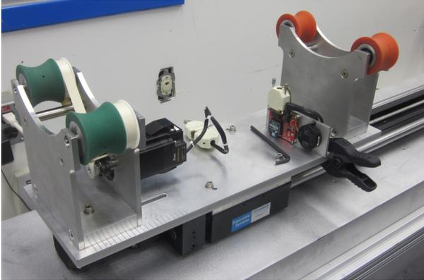
Figure 5: Cavity support, rotation and translation unit.
