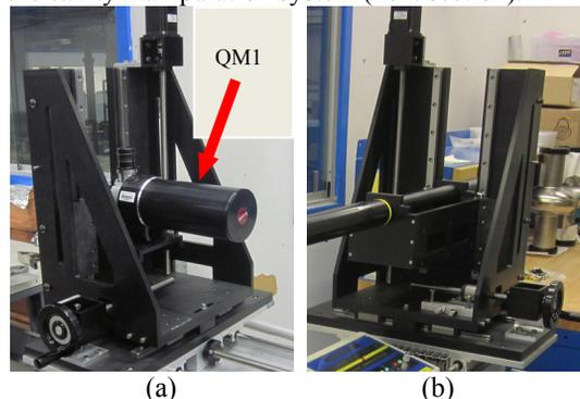
Figure 4: Positioning system of the Questar QM1 (a) and the mirror-bearing tube (b).
