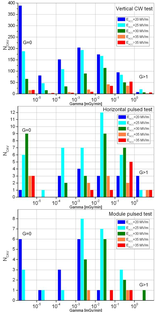
Figure 2: 9-cell SRF accelerating cavities tests at DESY: gamma radiation measurements statistics.
