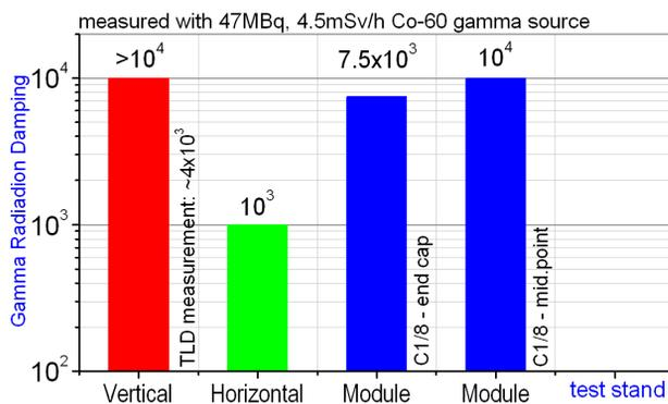
Figure 4: Gamma radiation damping measurements.
