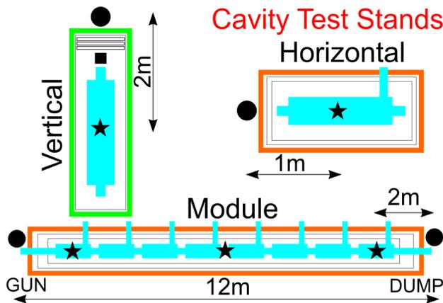
Figure 1: Cavity test stands gamma sensors (black orbs) and test Co-60 source (black stars) positions.
