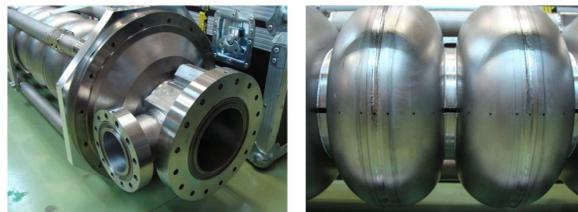
Figure 2: Detailed view of main acceleration cavities, input port and eccentric fluted beam pipe (left) stiffen rings (right).
