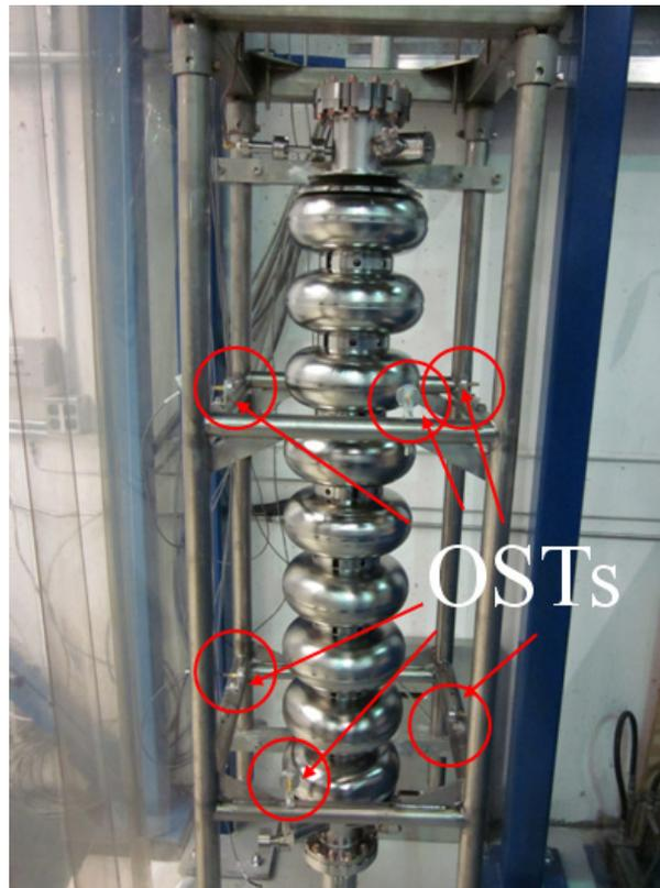
Figure 1: For the standard ILC RF test 8 OSTs are attached to the standard JLab cage around the cavity. Two more OSTs are behind the cavity and cannot be seen on this picture.
