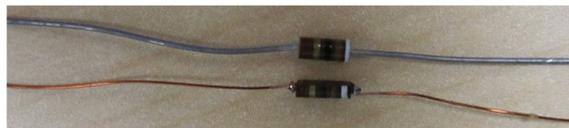
Figure 1: Preparation of AB100Ω resistors for arrays. The top is the original and the bottom is modified for the arrays. See description in the text.
