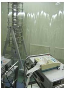
Figure 7: Particle count measurement in the cavity assembly area.
