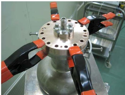
Figure 10: Clamping of the MO flanges.
