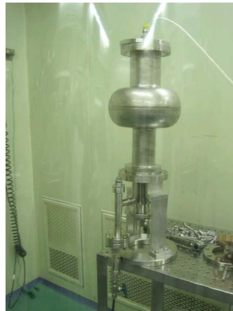
Figure 13: Cavity assembly using clean air flow.
