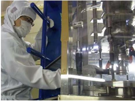
Figure 5: Window at the clean box to access the bottom valve.
