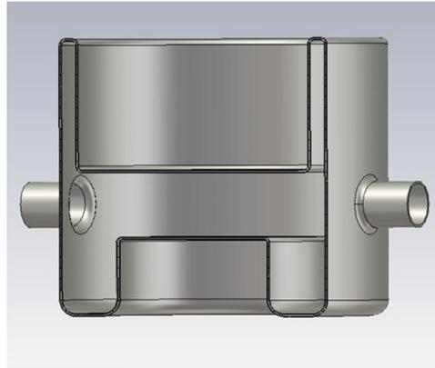
Figure 1: Concept model of QW crab cavity.
