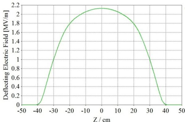
Figure 6: Deflecting electric field along the beam axis.
