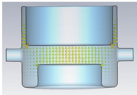
Figure 2: Electric field of the fundamental mode in the symmetric plane.
