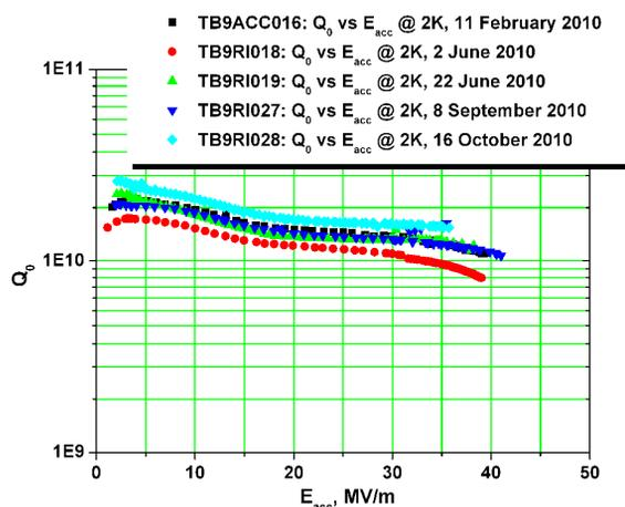
Figure 1:  $Q_0$  vs  $E_{acc}$  for five RI cavities tested at Jefferson Lab in 2010 are plotted in this picture. All cavities met ILC vertical acceptance test specification.
