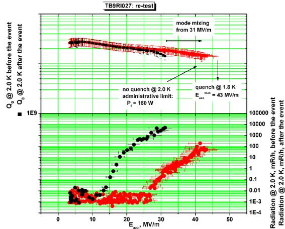
Figure 4: TB9RI027  $Q_0$  and radiation vs  $E_{acc}$  results before and after field emission event at  $T_{LHe\ bath} = 1.8$  K. The red squares in the upper plot are  $Q_0$  vs  $E_{acc}$  measurements and the red circles in the lower plot show radiation vs  $E_{acc}$  before the field emission event. The black squares in the upper plot are  $Q_0$  vs  $E_{acc}$  measurements and the black circles in the lower plot show radiation vs  $E_{acc}$  after the field emission event.
