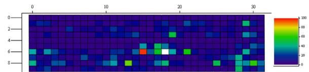
Figure 10: Temperature map of TB9RI027 after re-HPR at  $E_{acc} = 44$  MV/m in the center cell. Neither original nor new quench location shows any outstanding heating.
