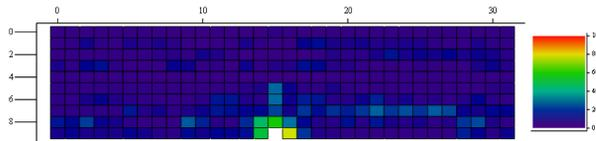
Figure 7: Temperature map of TB9RI027 after the field emission event at  $E_{acc} = 41$  MV/m. A clear field emission preheating pattern can be seen on this temperature map.
