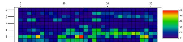
Figure 5: Temperature map of TB9RI027 at  $E_{acc} = 41$  MV/m before the field emission event. No indications of outstanding heating is present on the temperature map.
