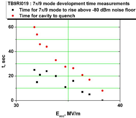
Figure 3: Mode-mixing measurements in TB9RI0019. Black dots show the time it took for the second mode to appear on the spectrum analyzer screen above the noise floor of -80 dBm. Red dots show the time it took for the cavity to quench during mode-mixing.
