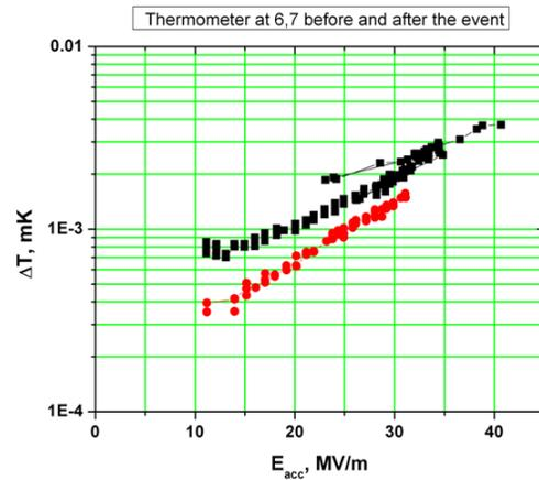
Figure 9: Preheating data from a thermometer close to original quench location. After field emission event thermometer still shows quadratic behavior at low field. The shift to a high temperature rise at low field indicates modification in surface resistance at the original quench location after field emission event.
