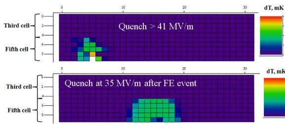
Figure 6: Temperature maps captured during repetitive quench of TB9RI027 before and after the field emission event. In the upper picture temperature maps of quench before field emission event is presented. In the lower picture temperature maps of quench after field emission event is presented.
