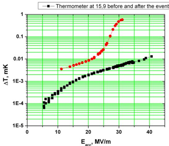
Figure 8: Preheating data from a thermometer close to new quench location. After field emission event thermometer field dependence changes from quadratic to a clear exponential behavior above  $E_{acc} = 25$  MV/m. Low field temperature rise is also different before and after field emission event, indicating an increase in low field surface resistance.
