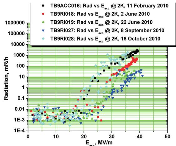
Figure 2: Radiation as function of field for five RI cavities tested at Jefferson Lab in 2010 is plotted in this figure. All cavities have shown field emission above  $1 \cdot 10^{-2}$  mR/h noise floor at accelerating gradients above 25 MV/m.
