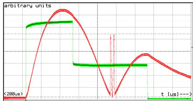
Figure 4b: PXFEL2\_1.HOM2.C2 signal – red, with cavity 2 partially detuned. Input RF power pulse – green.
