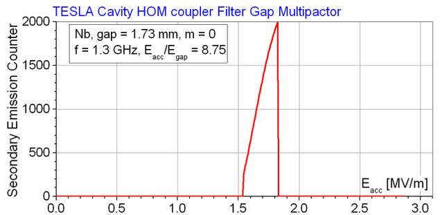
Figure 7: 1.3 GHz TESLA type cavity HOM coupler rejection filter gap analytical multipacting simulation.
