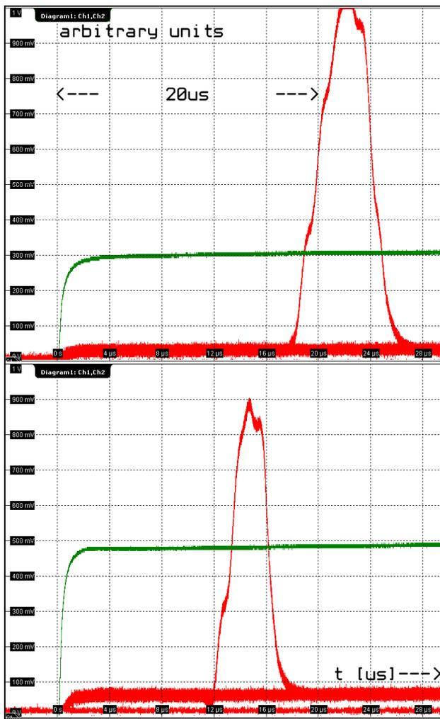
Figure 3: RF power change 170kW / 370kW, 100µs RF pulse – green, PXFEL3.C2.HOM1 pulse – red.
