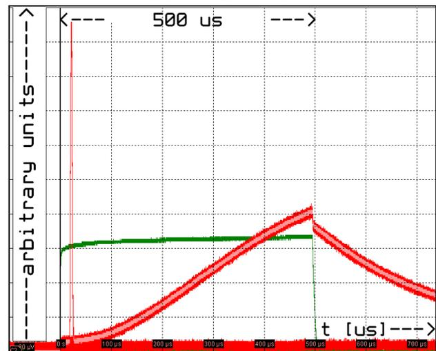
Figure 2: Anomalous peak with 500μs / 170kW RF pulse - green (21 MV/m). PXFEL3.C2.HOM1 pulse – red, measured with an RF diode.
