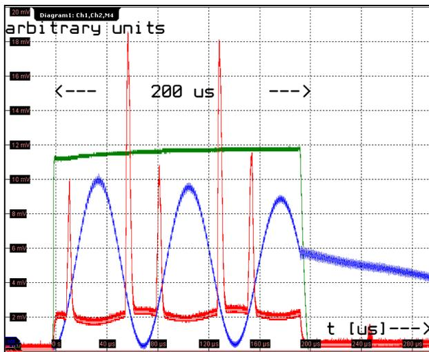
Figure 4a: PXFEL3.HOM1.C2 signal with cavity 2 partially detuned – red, blue – cavity probe signal.
