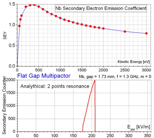
Figure 6: Flat gap multipacting simulation with niobium.
