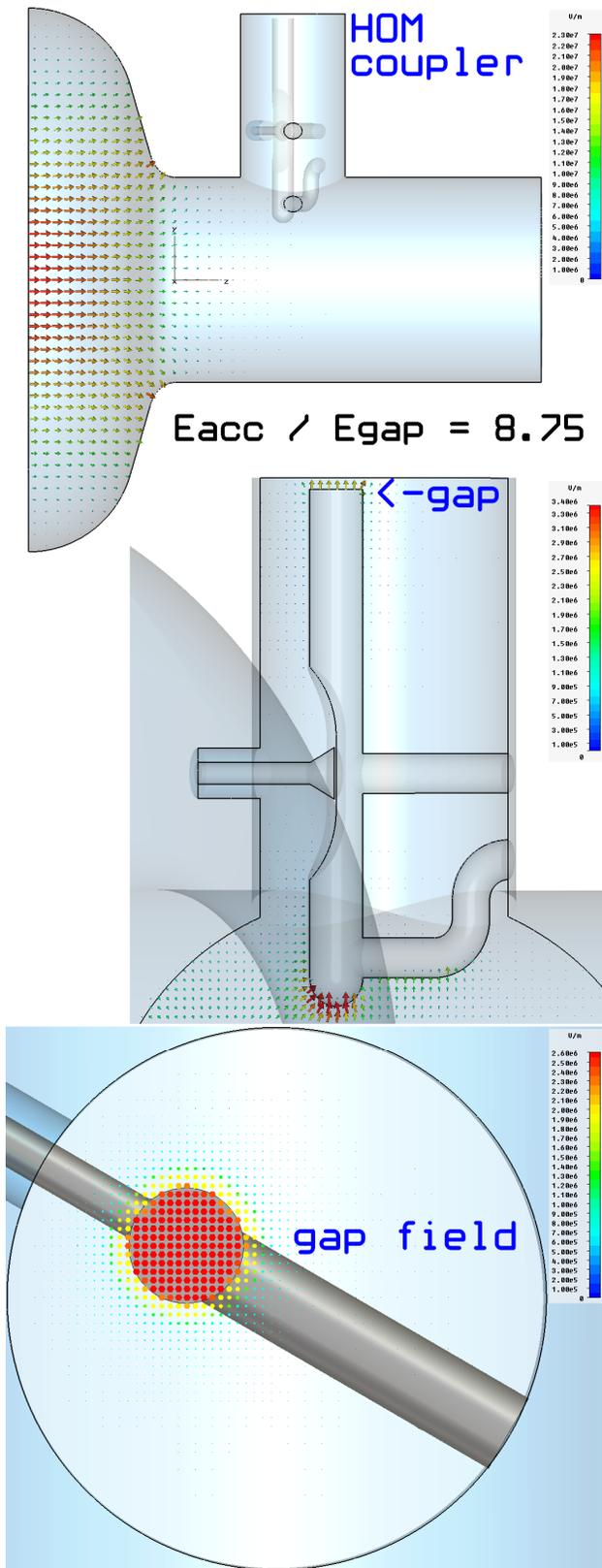
Figure 5: Cavity RF field simulation (CST Microwave Studio).
