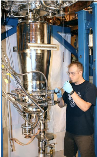
Figure 1: Prototype 72 MHz quarter-wave cavity with 4 kW power coupler and fast and slow tuners.
