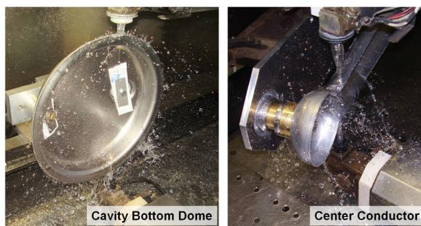
Figure 4: Wire electrical discharge machining (EDM) used to trim niobium cavity subcomponents.
