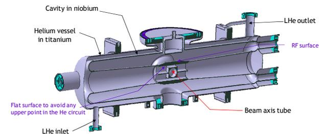
Figure 3: Final drawing of the HWR prototype.
