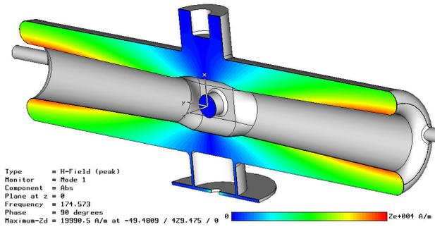
Figure 6: Integral of magnetic field inside the cavity.
