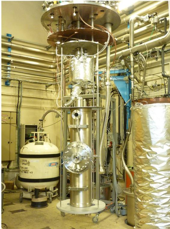
Figure 4: HWR prototype preparation for tests in vertical cryostat.
