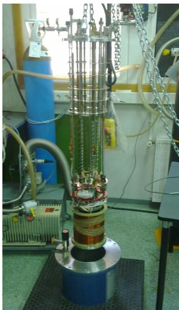
Figure 9: Solenoid prototypes preparation for tests in vertical cryostat.
