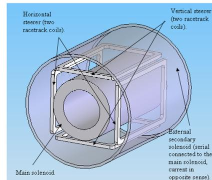
Figure 8: Coils configuration layout.
