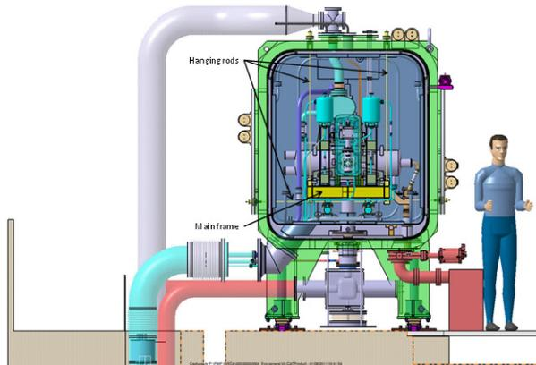
Figure 10: front view of the SRF Linac with its support, hanging rods and internal piping for cooling.
