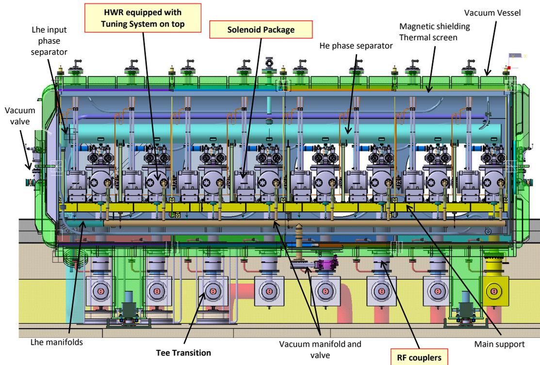
Figure 2: General layout of the LIPAc cryomodule.
