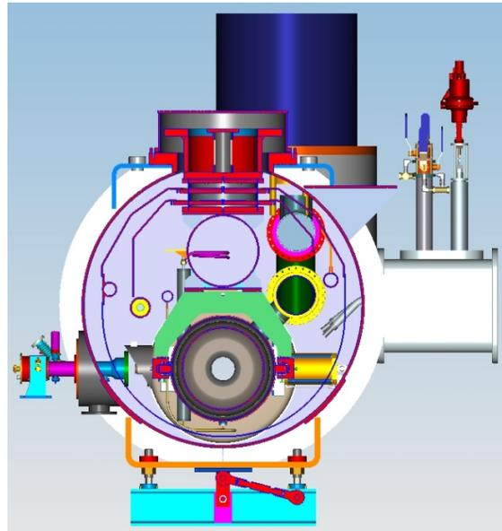
Figure 5: Cross section of 650 MHz cryomodule concept.
