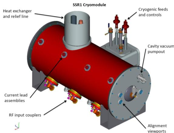
Figure 4: 325 MHz cryomodule concept.
