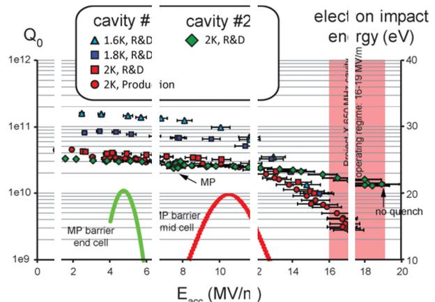
Figure 3: Test results from the JLab prototype cavities. Cavity #2 exceeded the specification at 16 MV/m. A multipacting simulation is shown on the secondary vertical axis.
