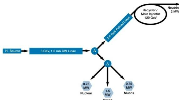
Figure 1: Schematic layout of the Project X accelerator complex.
