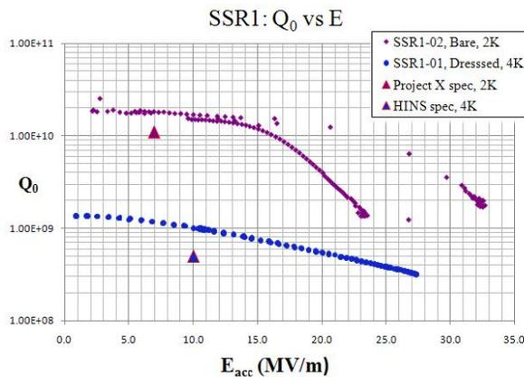
Figure 2: Performance of SSR1 cavities in bare (purple) and dressed (blue) cavity tests, at 2K and 4.2K, respectively, exceeded the specifications, shown by the purple and blue triangles, respectively, by a large margin.
