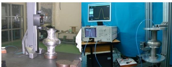
Figure 3: a) Mechanical measurement and b) RF measurement
