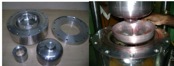
Figure 1: a) Forming tool and b) Forming of the half cell.
