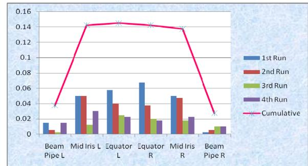
Figure 4a: Plot of material removed during CBP.
