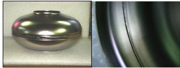
Figure 7: a) Half cell assembly with equator welded from both sides and b) Inner equator weld bead.
