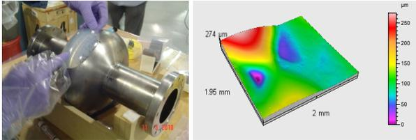
Figure 5: a) Cavity moulding and b) Profilometry plot of weld bead.
