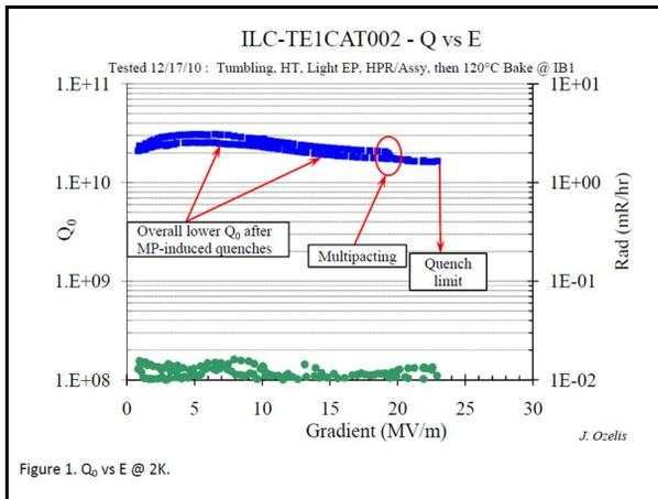
Figure 6: Q vs E plot of TE1CAT002.
