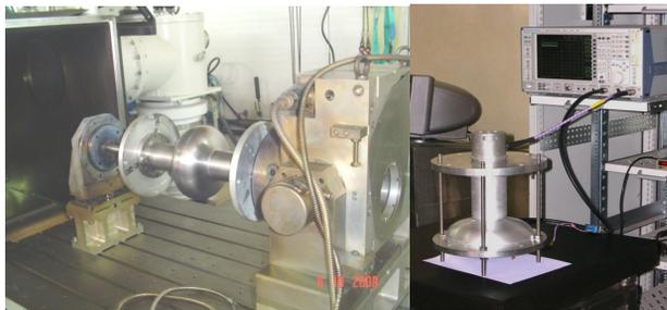
Figure 2: a) Electron beam welding setup and b) RF measurement of welded half cell assembly.
