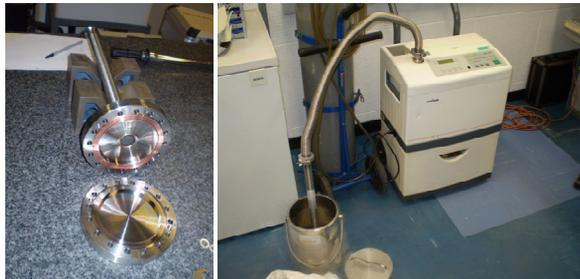
Figure 26: Ti6Al4V and 316LN CF flanges with OFE copper RF gasket tested at liquid nitrogen temperature.
