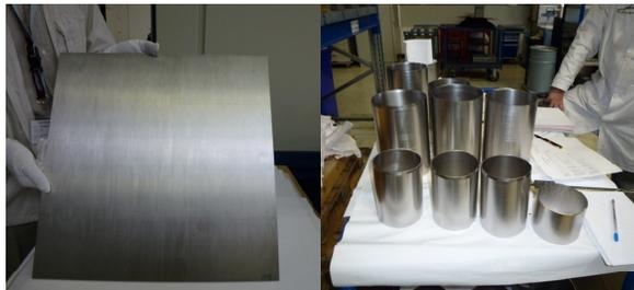
Figure 7: High purity niobium sheets and tubes.
