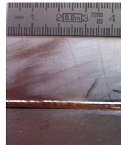
Figure 28: Surface features of Nb/304L joints electron beam welded with copper transition.
