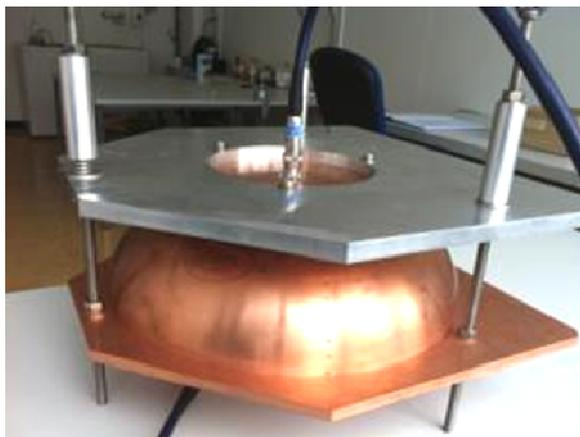
Figure 13: RF measurement of a copper half-cell.
