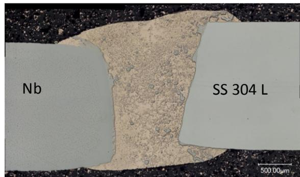
Figure 29: Macrostructure of cross section of weld.
