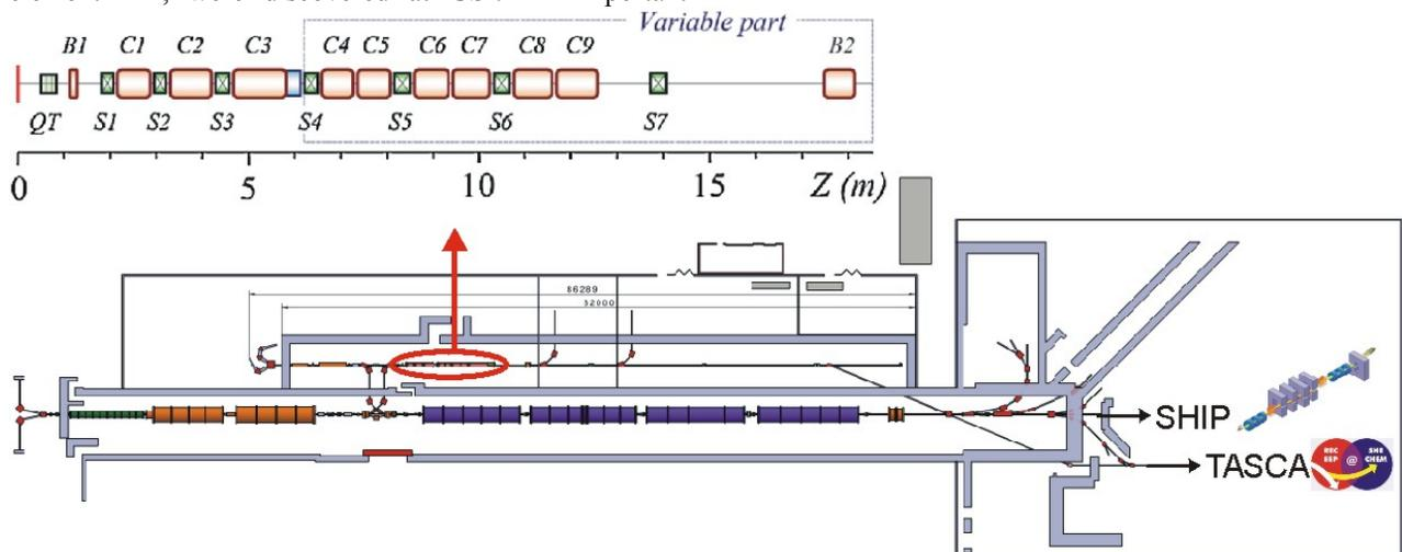
Figure 1: Draft layout of the future GSI accelerator facility with the integrated cw-LINAC in parallel to the existing UNILAC (Ci = Cavity, Bi = (Re-)Buncher, Si = Solenoid, QT = Quadrupole-Triplet). The cw-LINAC should provide SHE-experiments like SHIP (Separator for Heavy Ion reaction Products) and TASCA (TransActinide Separator and Chemistry Apparatus) with beam.
