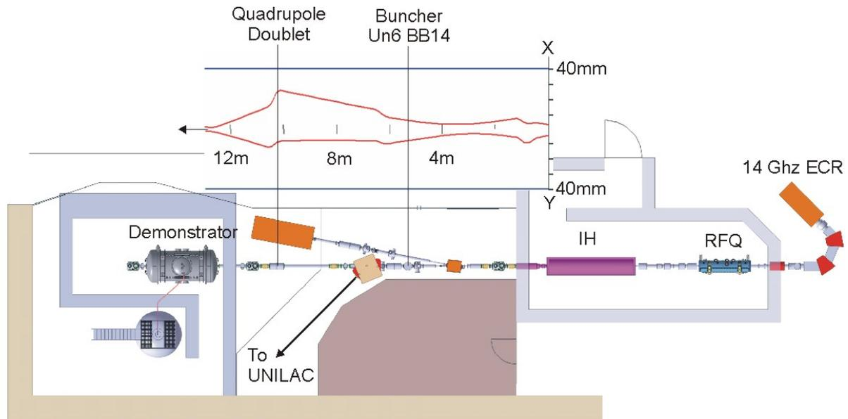
Figure 4: The existing HLI should be used as an injector for the cw-LINAC demonstrator. In longitudinal plane the existing buncher UN6BB, in transverse plane an additional quadrupole doublet should be used to match the beam to the demonstrator.
