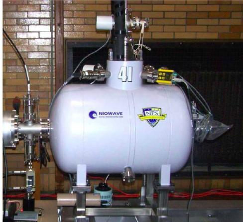
Figure 11: The fully assembled NPS/Niowave 500 MHz gun.
