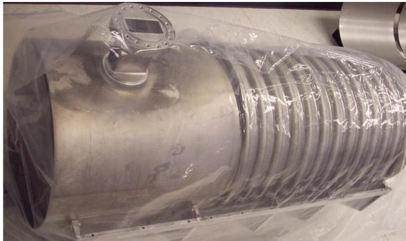
Figure 7: The 56 MHz QWR assembled outer conductor at Niowave.
