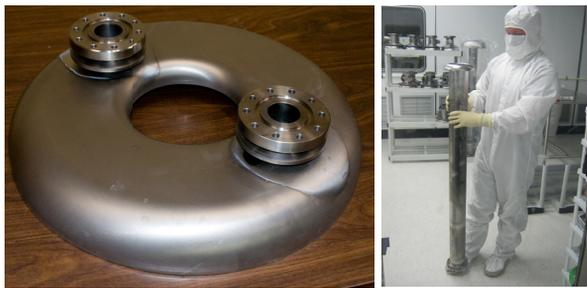
Figure 10: Parts of the 28 MHz accelerating cavity under fabrication at Niowave. Left: the end wall with coupling ports. Right: the beam pipe with nose-cone.
