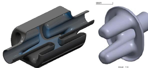
Figure 6: Design of a 4-rod superconducting crabbing/deflecting cavity.
