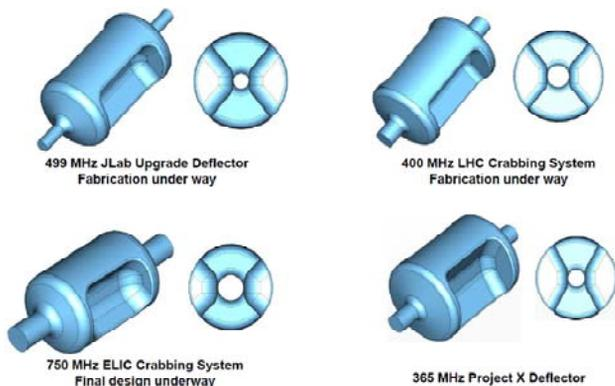
Figure 12: Parallel-bar cavities for several deflecting and crabbing applications.
