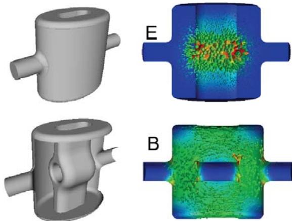
Figure 8: “Half-wave” resonator operating in a TE11-like mode.
