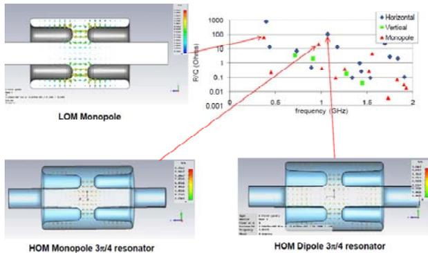
Figure 7: Lower-order and higher-order modes of a superconducting 4-rod cavity.
