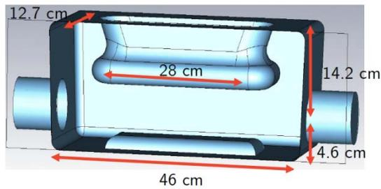
Figure 16: 400 MHz quarter-wave geometry for the LHC crabbing system.
