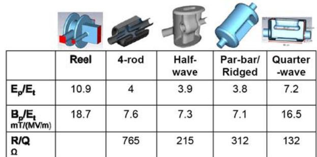
Figure 18: Electromagnetic properties of a number of 400 MHz crabbing cavities.
