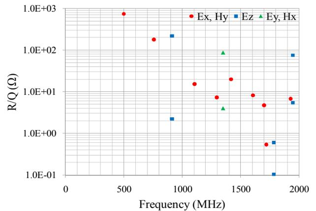
Figure 13: Higher-order modes of a 499 MHz parallel-bar cavity.
