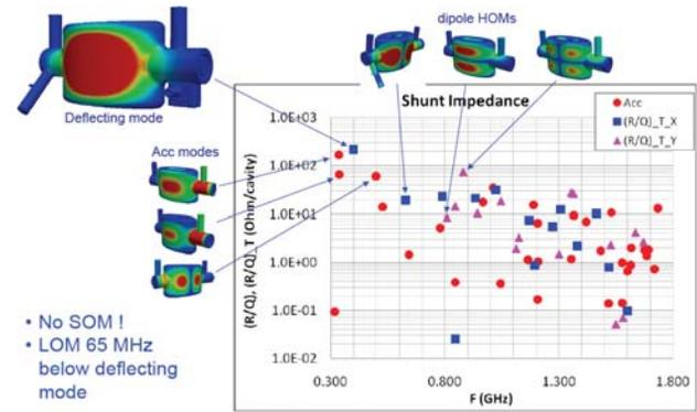
Figure 9: Lower-order and higher-order mode properties of the SLAC “half-wave” cavity.
