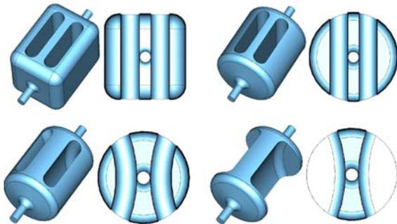
Figure 11: Evolution of the design of parallel-bar cavities.
