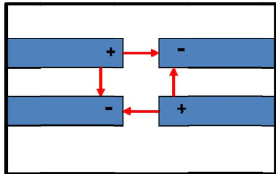
Figure 5: Mode of operation of a 4-rod cavity.
