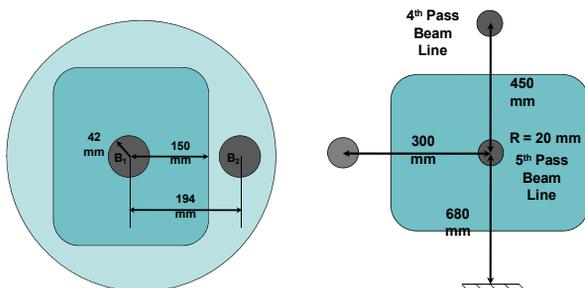
Figure 3: Dimensional constraint for the 400 MHz LHC crabbing system (left) and the JLab Upgrade 499 MHz deflecting system (right).
