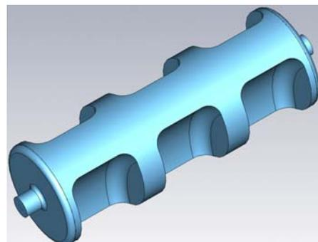
Figure 15: 3-cell version of the cavity in Fig. 12.
