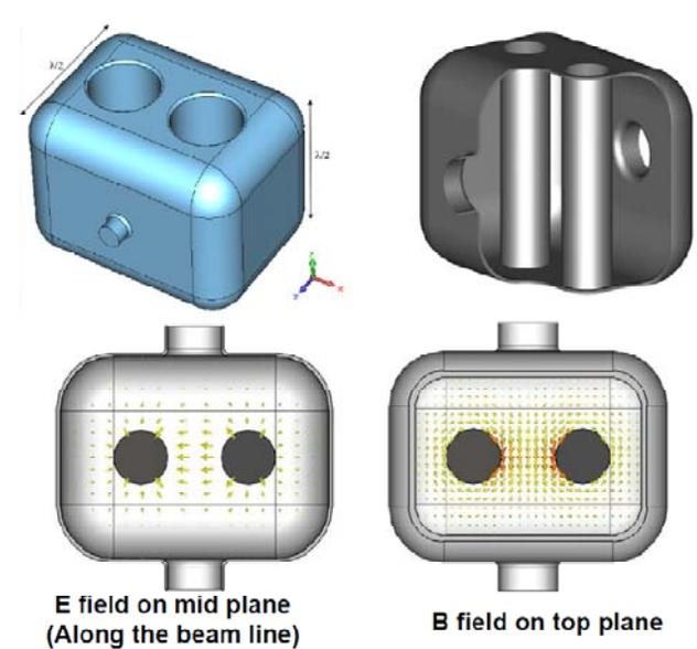
Figure 10: Concept for the parallel-bar deflecting/crabbng cavity.
