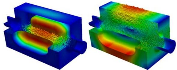
Figure 14: 400 MHz ridged-waveguide cavity [11].
