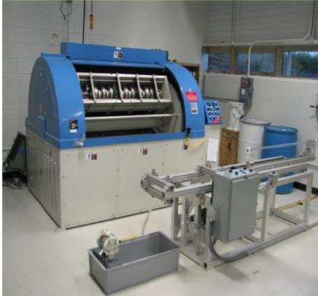
Figure 10: Centrifugal Barrel Polishing (CBP) machine in use at FNAL. Identical machines have been acquired by Cornell and JLab.
