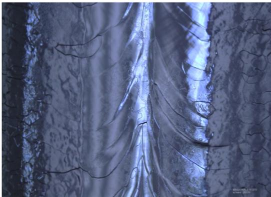
Figure 6: Area of cavity TB9RI024 which was the site of a 29MV/m quench. No discernable “feature” is seen.
