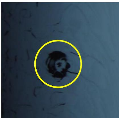
Figure 7: Feature with a diameter of ~1000µm found on cavity TE1AES004 which quenched at 40MV/m, but not at the location of this feature.
