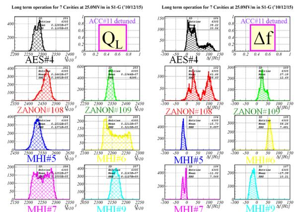
Figure 21: The distributions of  $Q_L$  and the detuning frequency during the long term operation for 7 cavities.
