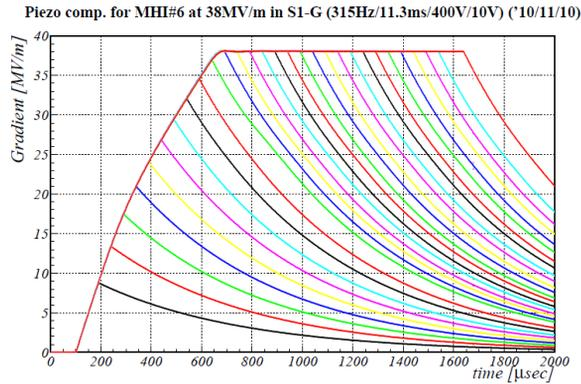
Figure 10: The example of the pulse shortening method. Each step is 50 µs.
