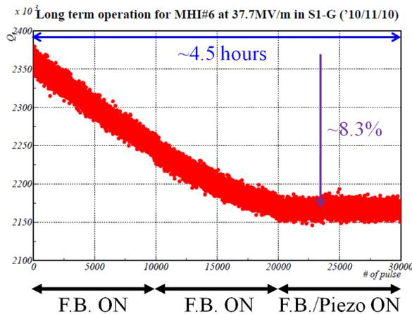
Figure 19: The trend of  $Q_L$  during the long term operation for MHI-06.
