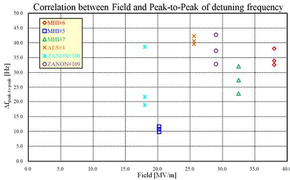
Figure 18: The correlation between the excursion peak-to-peak of the detuning frequency at flat-top and field. The best three results are shown here.
