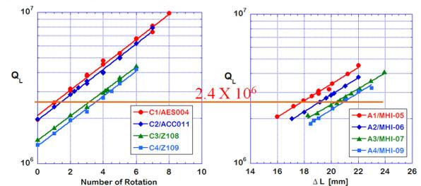
Figure 7: The results of the drive test for the variable coupling of the power couplers.
