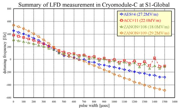
Figure 12: The result of LFD measurement at the maximum gradient for every cavity.
