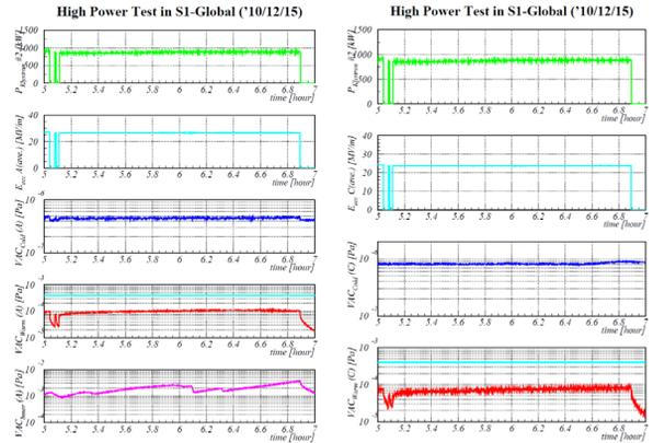
Figure 23: The trend of helium level, helium pressure, helium flow and vacuum during the long term operation (17:00-19:00). 12:00-19:00 (top-left) and 17:00-19:00 (others). The vacuum level at three locations for Cryomodule-A (left) and two locations for Cryomodule-C (right) are shown in the bottom figures.
