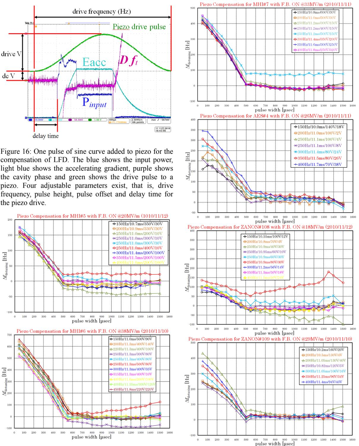
Figure 17: Results of the compensation by piezo for 6 cavities. Adjustable parameters in black framework show drive frequency, delay time, pulse height and pulse offset for sine curve pulse (from left to right).
