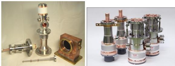
Figure 2: TTF-III (left) and STF-II (right) couplers.
