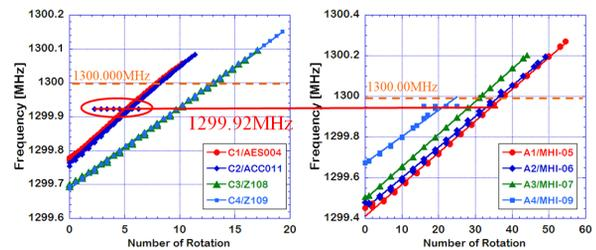
Figure 6: The result of the drive test for the motor tuner at low power. The tuner of ACC011 did not work at 2K, and MHI-09 could not be set to 1300.000 MHz.
