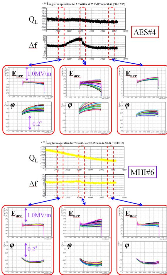
Figure 22: The superimposed RF pulses at the flat-top for three periods during the long term operation.
