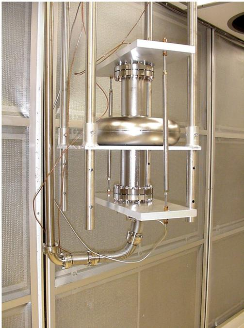
Figure 1: Cavity assembled to test stand; as discussed below, an attempt was made to stiffen up the cavity with Ti rods.
